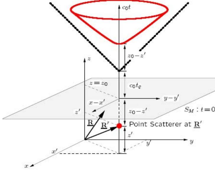
Figure 1: Diffraction surface (red) of a point scatterer (red dot)
