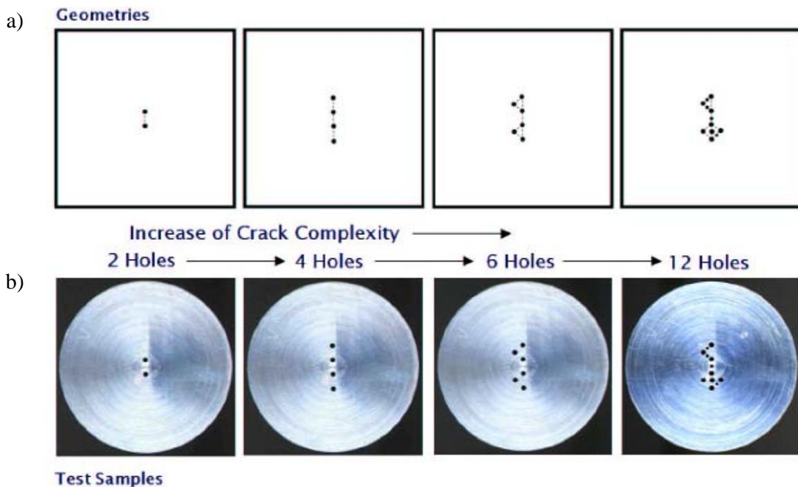
Figure 3: The stepwise increase of crack complexity: a) samples geometries of two, four, six and twelve holes, b) aluminium samples
