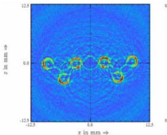
Figure 4: SAFT reconstruction of the multi-pulse-echo data set
