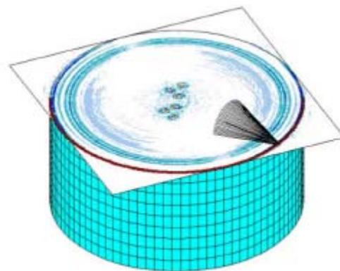
Figure 5: SAFT reconstruction embedded in the 3-D geometry of the test sample
