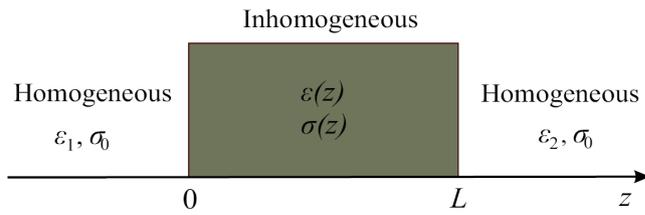
Figure 7: Geometry of the inhomogeneous slab
