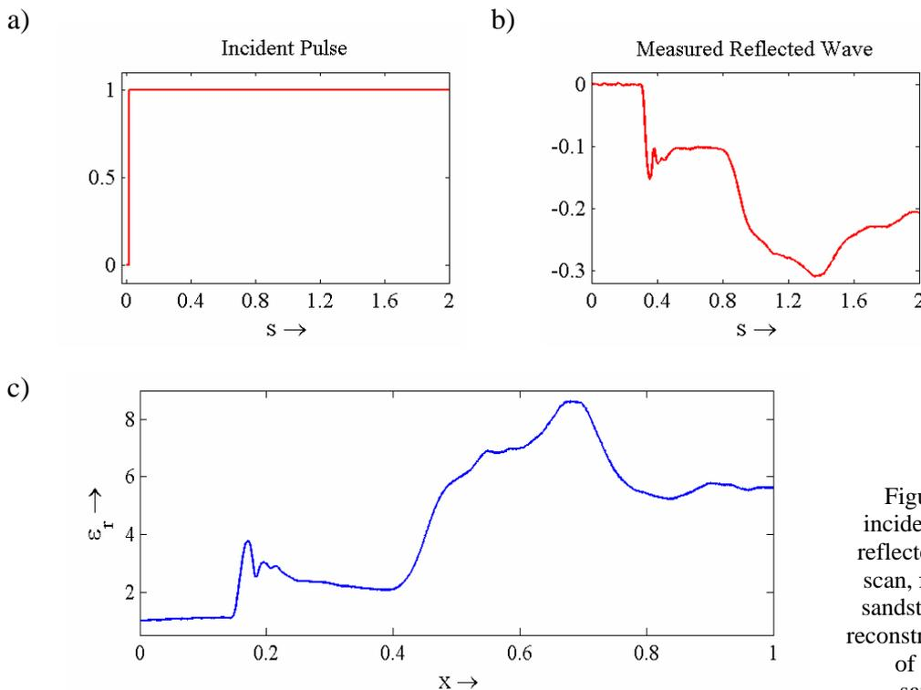
Figure 13: a) incident wave, b) reflected wave, A-scan, from a lime sandstone slab, c) reconstructed profile of the lime sandstone
