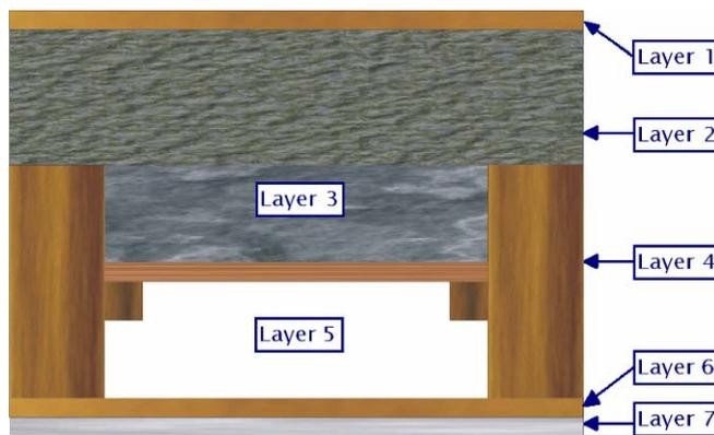
Figure 9: Geometry of the multi-layered test slab
