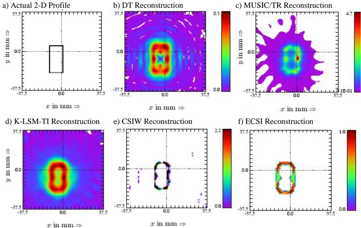
Figure 2: Reconstruction results for a centred metallic rectangular cylinder (PEC) target of electromagnetic Fresnel data with TM polarization: a) Actual shape and position, b) DT reconstruction, c) MUSIC reconstruction, d) K-LSM-TI reconstruction, e) CSIW reconstruction, f) ECSI reconstruction. The results in b)-d) are obtained using the 16 GHz data. The results in e) and f) are achieved using the frequency-hopping approach with the data at 4, 8, 12 and 16 GHz.
