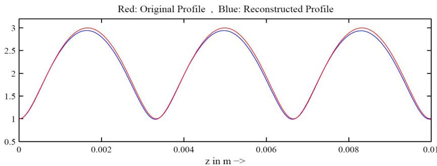
Figure 8: Original relative permittivity profile of the slab (red) and reconstructed profile (blue)
