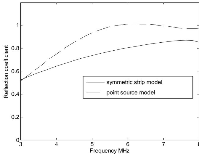
**Figure 5** Comparison of results from the 'hybrid' model and symmetric strip model at normal incidence for an array of slit scatterers (30% contact)
