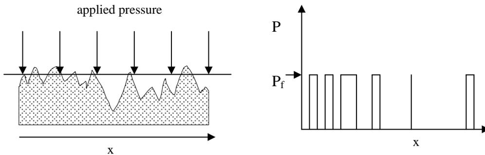
**Figure 1** Plastic random surface contact model to predict the interfacial geometry
