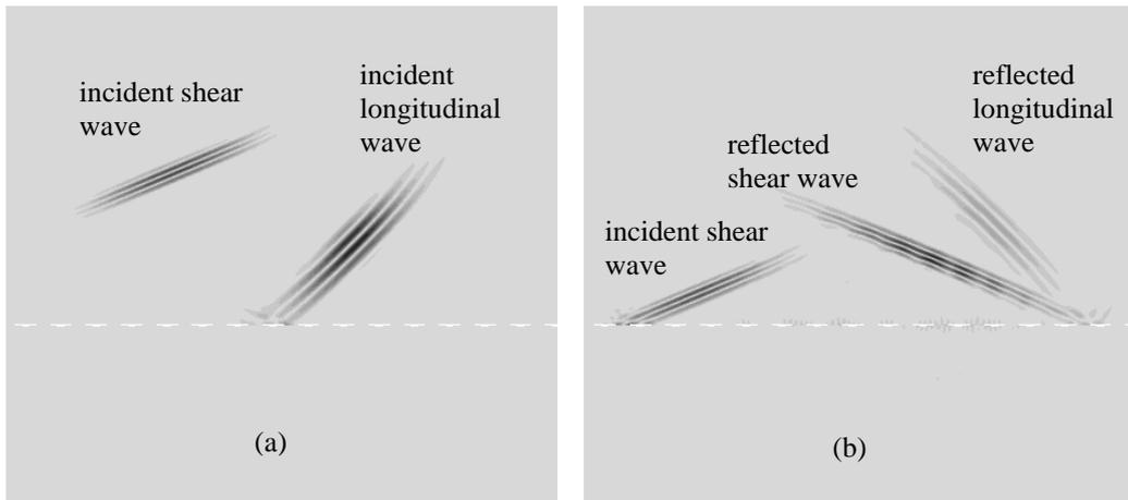
**Figure 7** (a) Incident wave and (b) reflected waves from the finite element model
