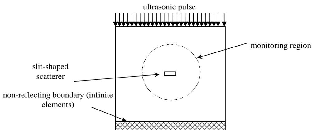
**Figure 2** Schematic diagram of single scatterer model
