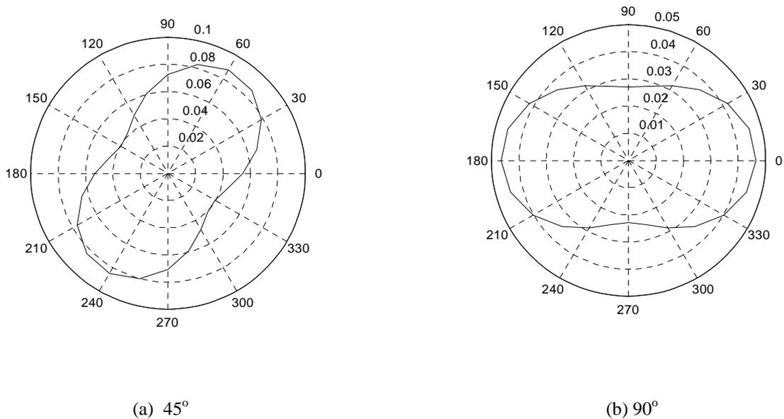
**Figure 3** Angular displacement and phase for a slit orientated at (a) 45° to the incident wave and (b) 90° to the incident wave
