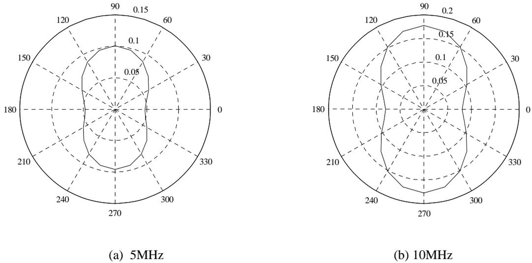
**Figure 2** Angular displacement for a slit-shaped scatterer (width 0.18mm) at 5 and 10MHz
