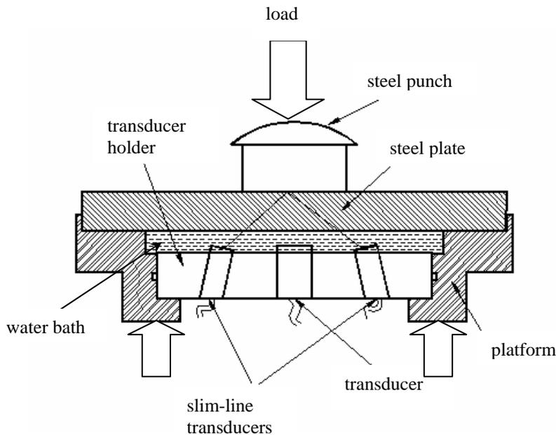
**Figure 8** Schematic diagram of the experimental apparatus oblique incidence
