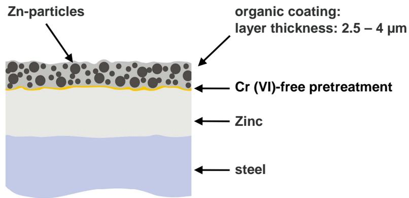
**Figure 1.** Principle of layer structure of a corrosion protection primer of the first generation
