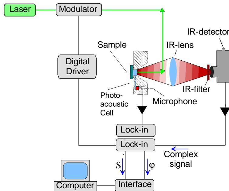
**Figure 3.** Schematic of the measurement device, enabling simultaneously IR radiometric and photoacoustic detection of thermal waves
