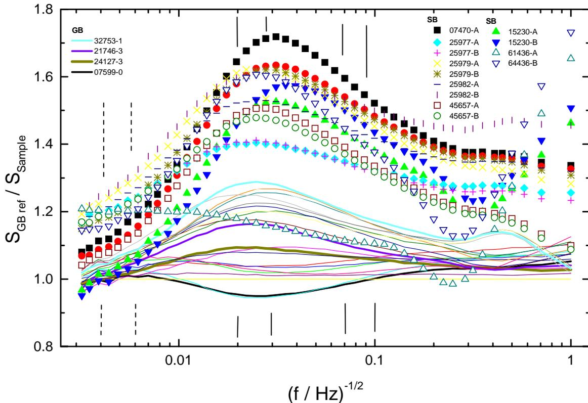
**Figure 9.** Inverse normalized modulated IR amplitudes  $S_{GBref}/S_{sample}$  versus the penetration depth of the thermal wave, using an arbitrary SB sample of good welding properties (GB 24127) as reference sample for normalization.
