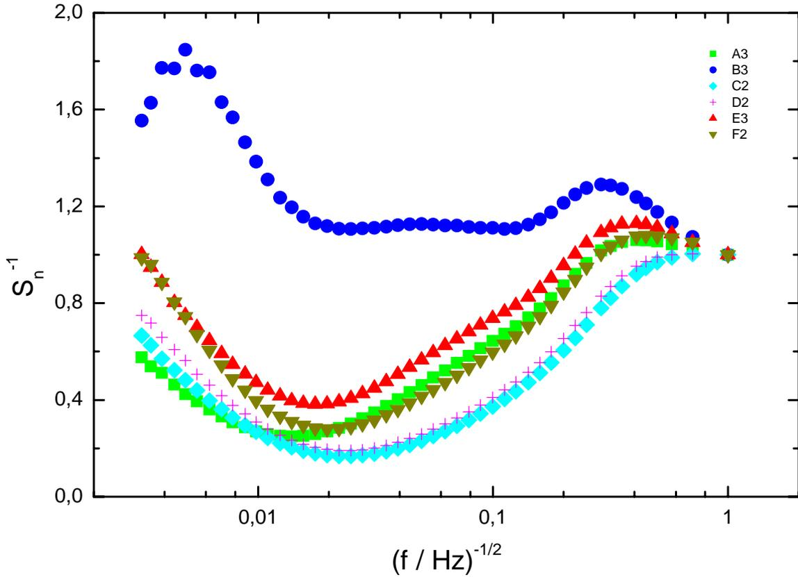
**Figure 6.** Inverse calibrated modulated IR amplitudes of the coated steel sheet test samples after additional normalization on the value of 1 at large penetration depths.
