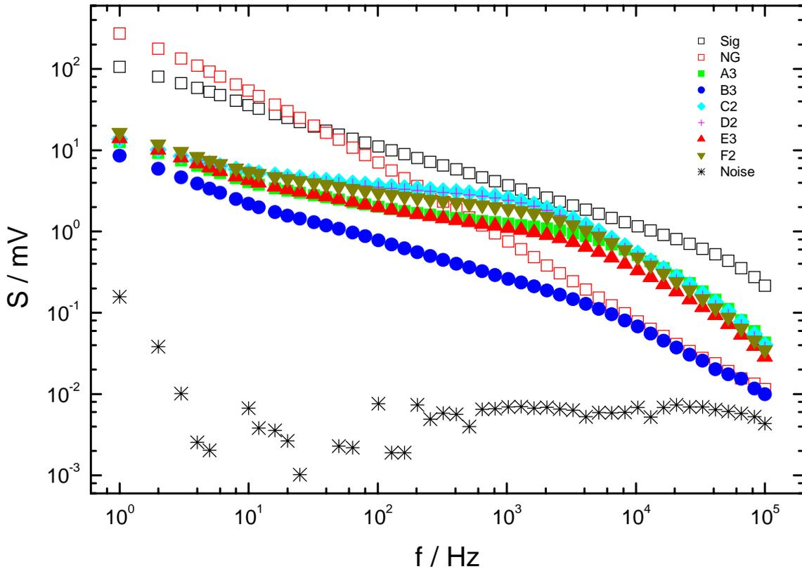
**Figure 4.** Modulated IR amplitudes measured as a function of the heating modulation frequency for coated steel sheet samples, in comparison with the noise signal (\*) and the reference signals measured for opaque homogeneous glassy carbon (Sigradur □) and semi-transparent neutral density glass (Schott NG1 □).
