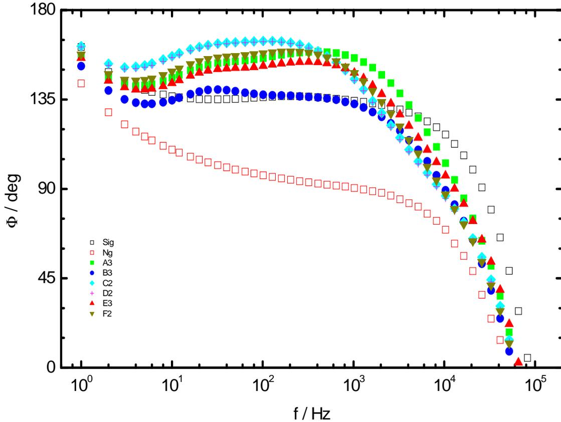
**Figure 5.** Modulated IR phases measured as a function of the heating modulation frequency for coated steel sheet test samples, in comparison with the reference signals measured for an opaque homogeneous sample of glassy carbon (Sigradur  $\square$ ) and a semi-transparent sample of neutral density glass (Schott NG1  $\square$ )
