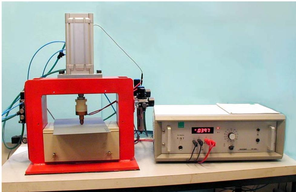
**Figure 2.** Laboratory system to measure the electrical resistance of spot-welded joints
