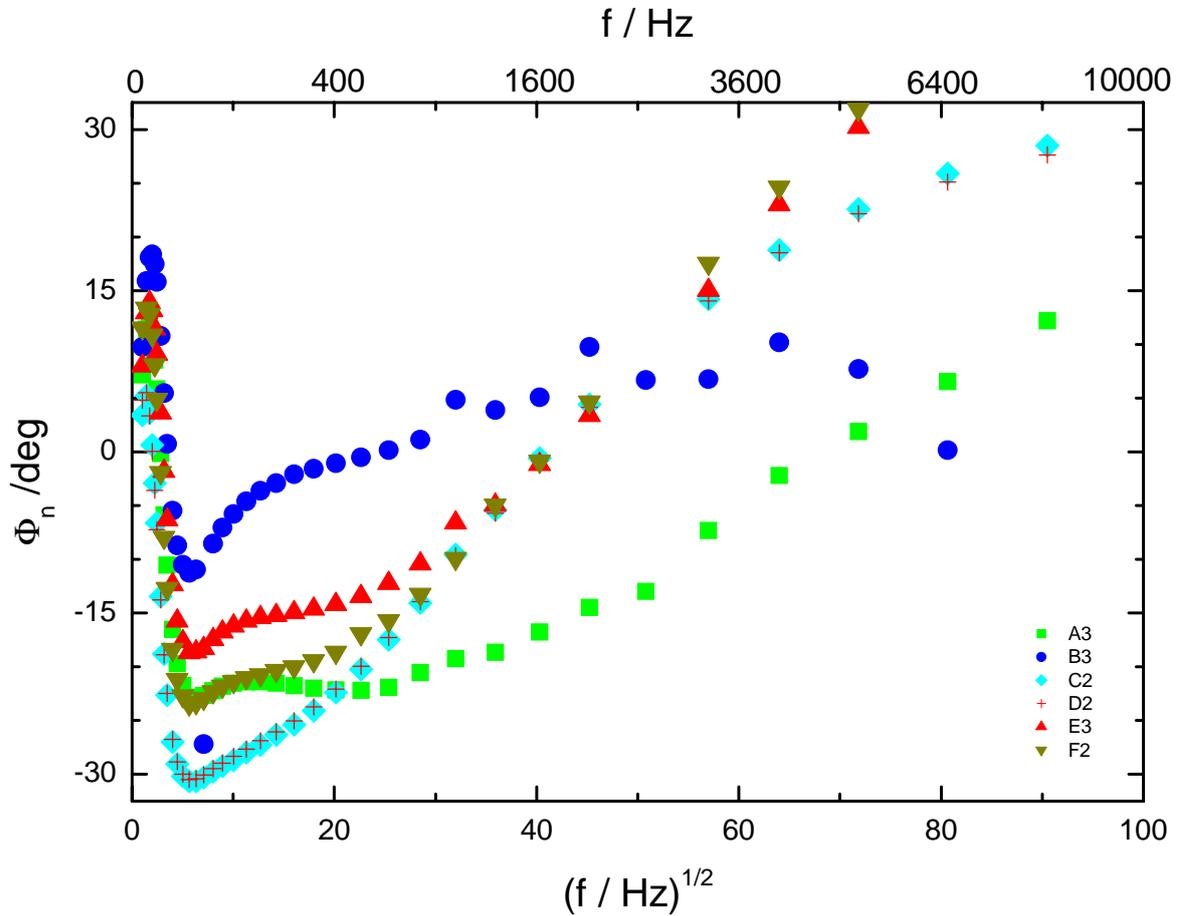
**Figure 7.** Inverse calibrated photoacoustic phases obtained for the coated steel sheet test samples
