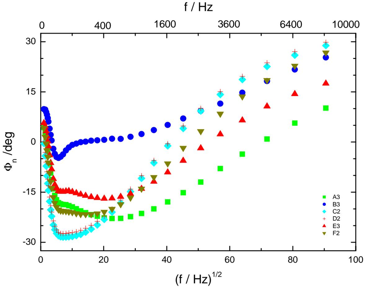
**Figure 8.** Inverse calibrated modulated IR phases obtained for the coated steel sheet test samples
