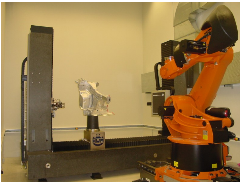
Fig. 4: CT system RayScan 200 XE inside of the shielding cabinet
