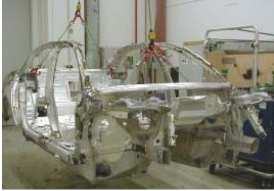
Fig. 1: Car body being cut into pieces for destructive testing
