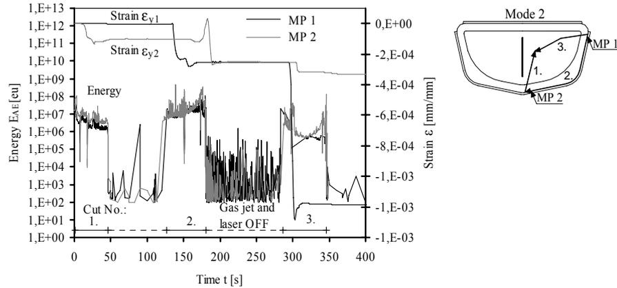
**Fig. 10:** Energy  $E_{AE}$  and strain  $\epsilon_y$  of right mud-guard as a function of time  $t$ , cutting mode 2.
