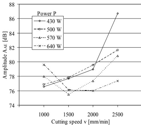
**Fig. 4:** Maximum amplitude  $A_{AE}$  of acoustic emission in laser cutting as a function of cutting speed  $v$  and laser-beam power  $P$ .
