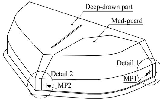
**Fig. 1:** Deep-drawn part; definition of measuring points.
