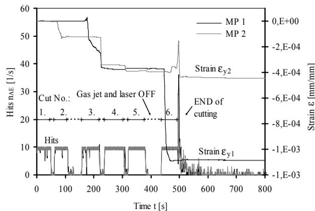
**Fig. 9:** Number of AE hits  $n_{AE}$  and strain  $\varepsilon_y$  of right mud-guard as a function of time  $t$ ; cutting mode 1.
