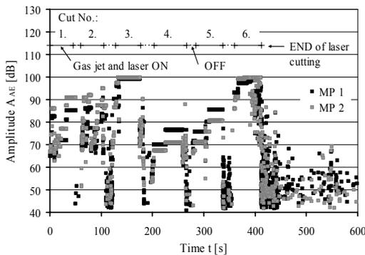
**Fig. 6:** Maximum amplitude  $A_{AE}$  of AE signals captured in certain time period during laser cutting.
