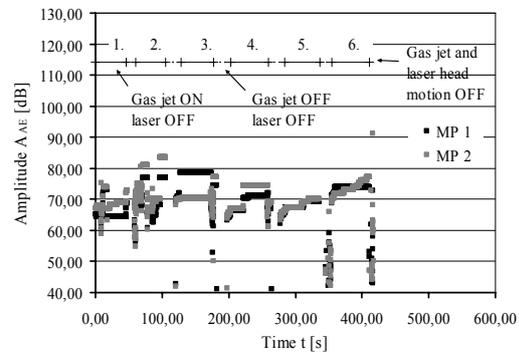
**Fig. 7:** Maximum amplitude  $A_{AE}$  of AE signals captured in certain time period during laser-head travel with just cutting-gas jet - no cutting.
