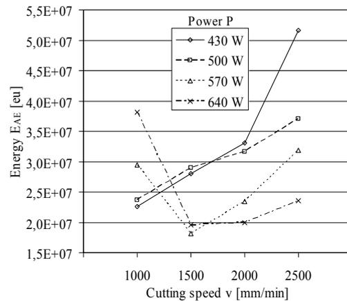
**Fig. 5:** Energy  $E_{AE}$  of acoustic emission in laser cutting as a function of cutting speed  $v$  and laser-beam power  $P$ .
