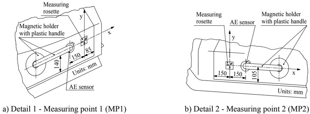
**Fig. 3:** Location of AE sensors and resistance measuring rosettes at deep-drawn part (details of Fig. 1).
