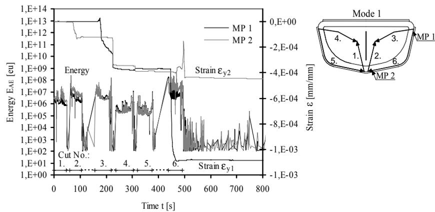
**Fig. 8:** Energy  $E_{AE}$  and strain  $\varepsilon_y$  of right mud-guard as a function of time  $t$ ; cutting mode 1.
