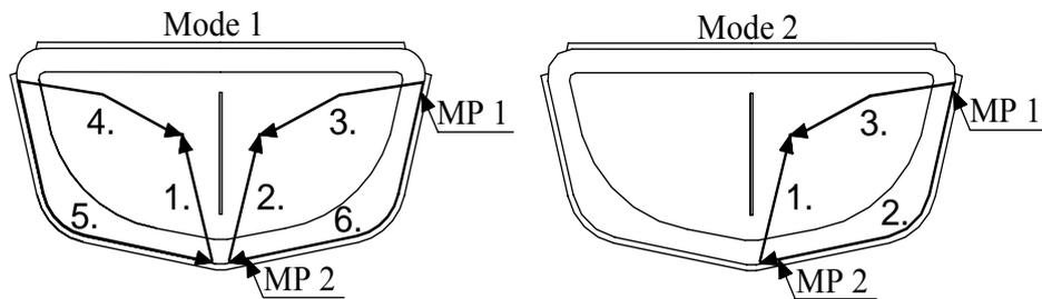
**Fig. 2:** Modes of cutting mud-guards out of deep-drawn part.
