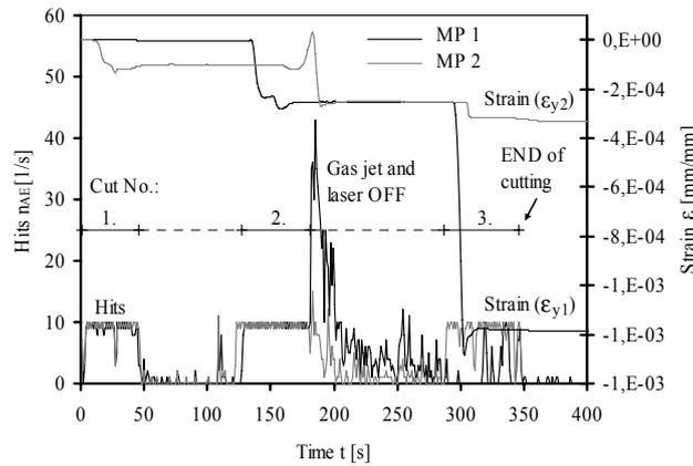
**Fig. 11:** Number of AE hits  $n_{AE}$  and strain  $\epsilon_y$  of right mud-guard as a function of time  $t$ , cutting mode 2.
