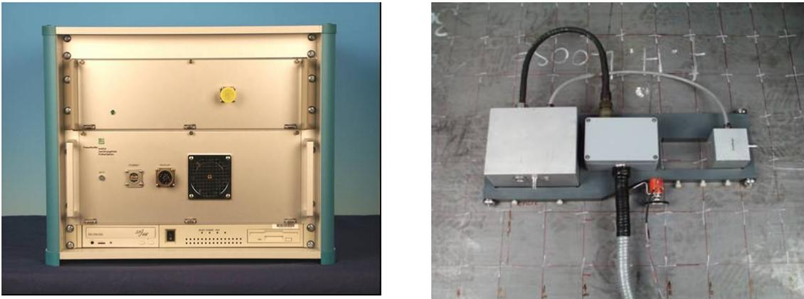
**Figure 7.** Combined 3MA+DM hardware unit (left), DM probe with transmitter and receiver(right)
