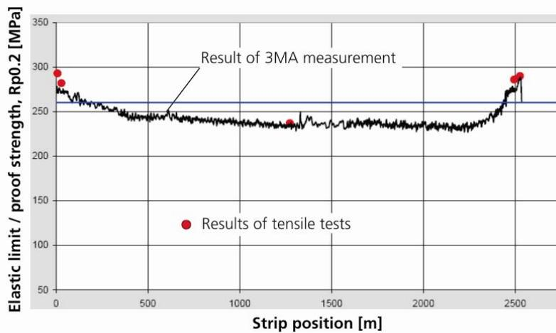
**Figure 2.** Continuous Rp0.2 measurement with 3MA on a steel strip with increased strength at the ends
