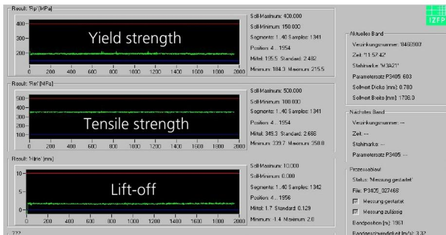
**Figure 4.** Online visualization of yield and tensile strength of a running strip
