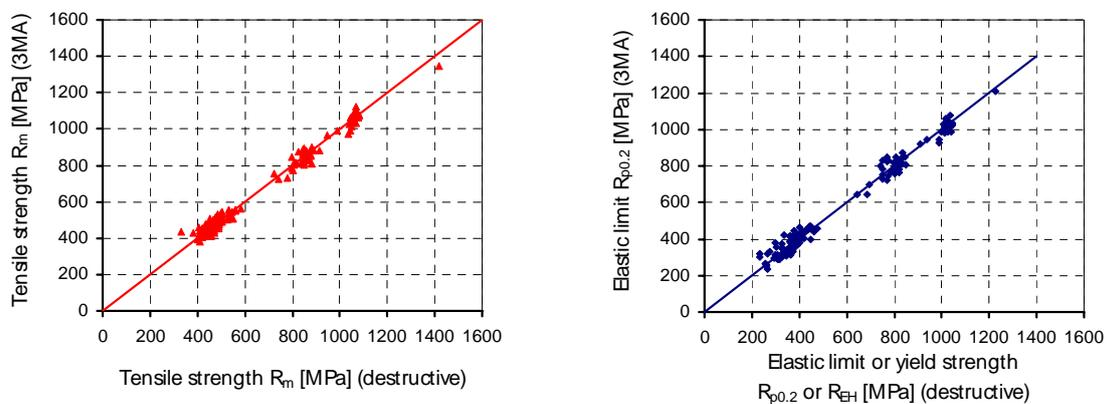
**Figure 6.** Non-destructively predicted tensile and yield strengths as a function of the destructively determined results
