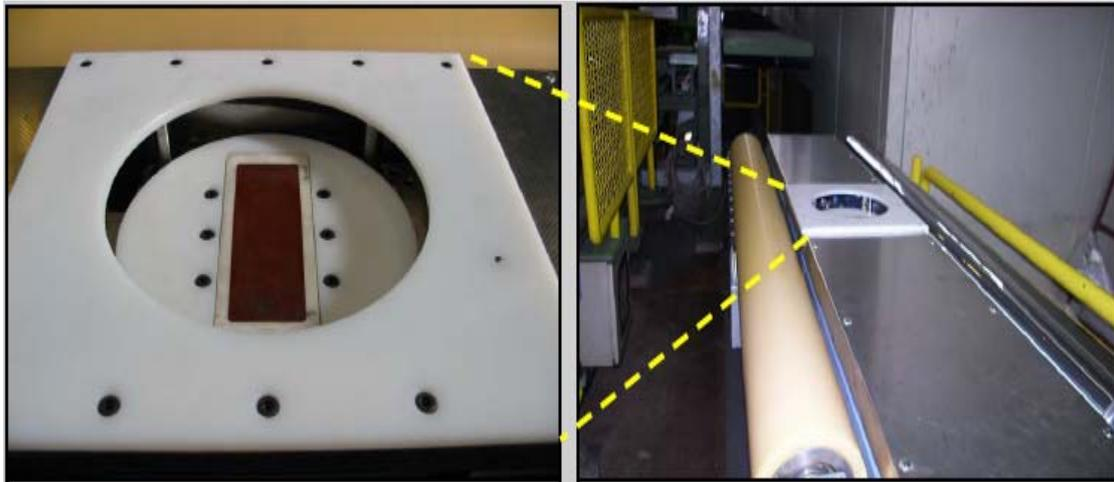
**Figure 3.** 3MA probehead holder and table carrier of the in-line steel sheet inspection system
