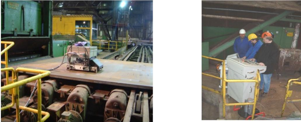
**Figure 5.** 3MA inspection trolley (left picture) and remote control desk (right picture)
