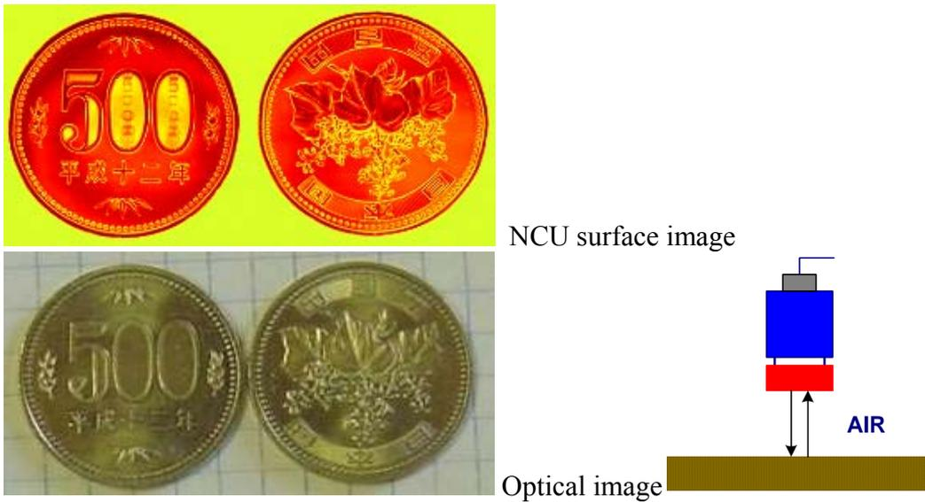
**Fig. 3** Pulse-echo schematic diagram and surface images of a Japanese 500 Yen coin characterized by very fine features. Compare the NCU and optical images
