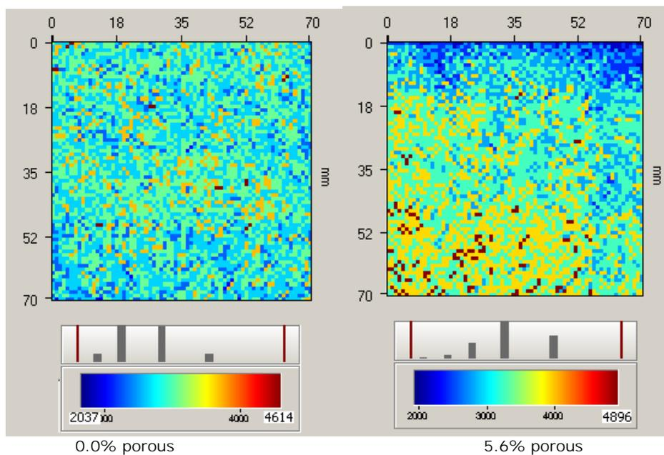
**Fig. 9** Data 70x70-mm distribution of the 1.0 MHz NCU velocity (m/s) versus 0.0% (left) and 5.6% (right) porosities for the 8-ply CFRP sample.
