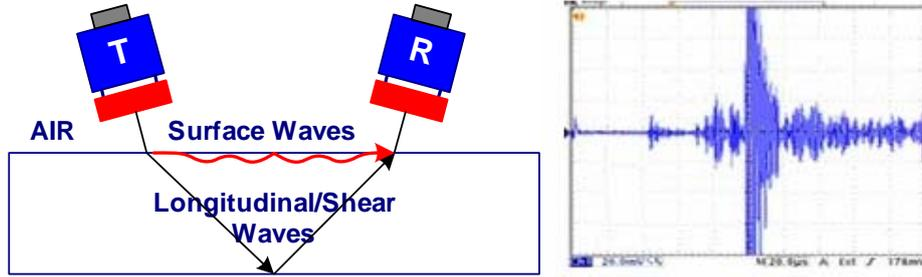
**Fig. 2** Pitch-catch schematic diagram and typical A-scan showing the appearance of surface and bulk waves in a 50 mm thick section of polystyrene.
