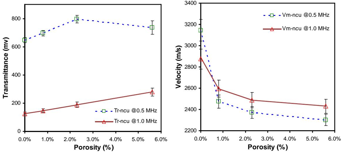
**Fig. 10** Typical relationship of the NCU relative transmittance (left) and velocity (right) versus porosity for 0.50 MHz and 1.0 MHz nominal frequencies in the 1.9 mm 8-plyes of CFRP samples.
