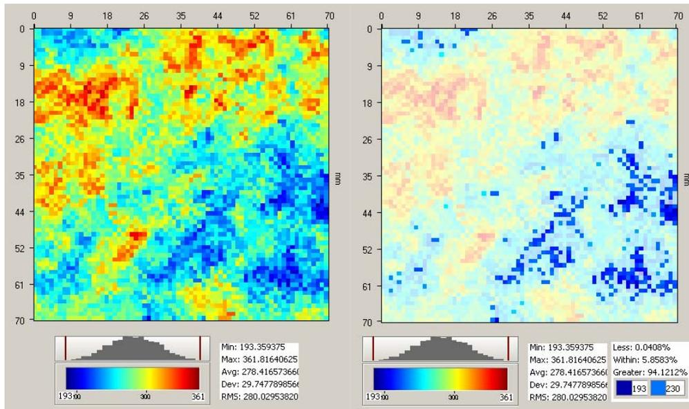
**Fig. 11** Spatial distribution of the porous regions in blue (right) for the 5.6% porosity, 8-plyes CFRP sample obtained by analysis of the Gaussian distribution of transmittance values, evaluated at 1.0 MHz. Using  $p \leq 0.10$ , the derived average porosity is 5.8% which includes the transmittance values of less than 193 mv and greater than 230 mv.
