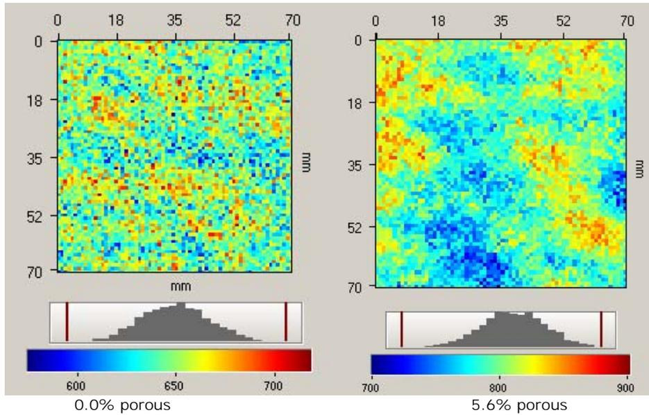
**Fig. 6** Data 70x70-mm distribution of the 0.5 MHz NCU relative transmittance (mv) versus 0.0% (left) and 5.6% (right) porosities for the 8-ply CFRP sample.
