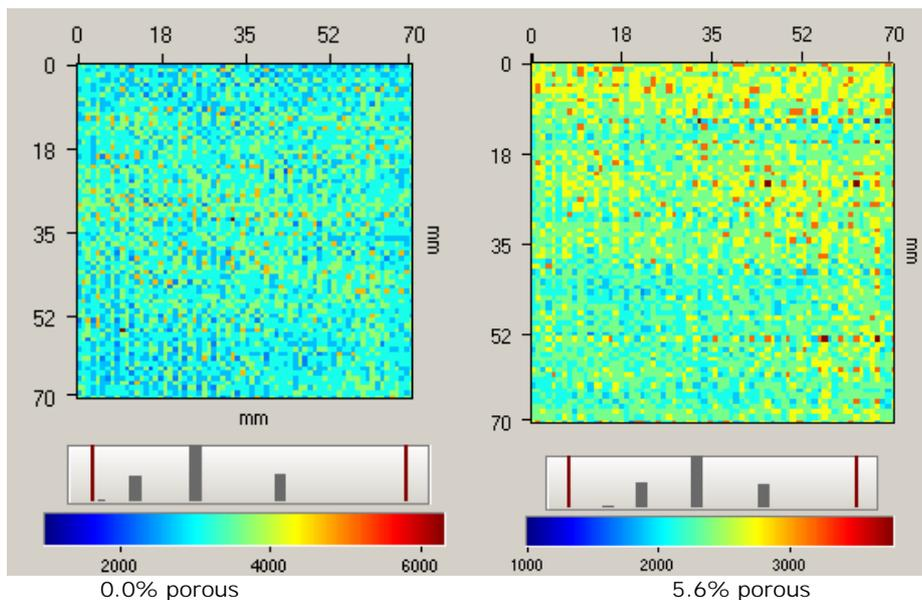
**Fig. 7** Data 70x70-mm distribution of the 0.5 MHz NCU velocity (m/s) versus 0.0% (left) and 5.6% (right) porosities for the 8-ply CFRP sample.
