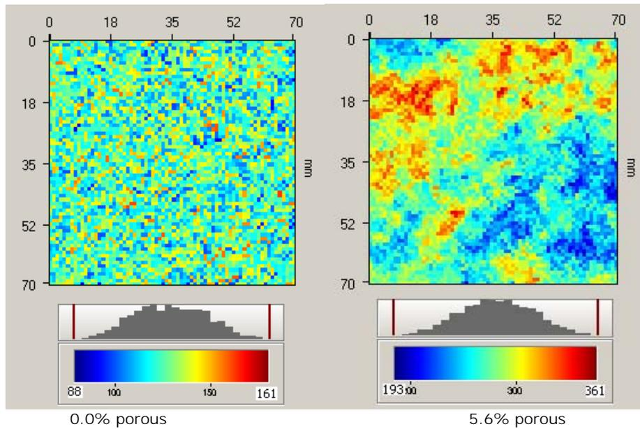
**Fig. 8** Data 70x70-mm distribution of the 1.0 MHz NCU relative transmittance (mv) versus 0.0% (left) and 5.6% (right) porosities for the 8-ply CFRP sample.
