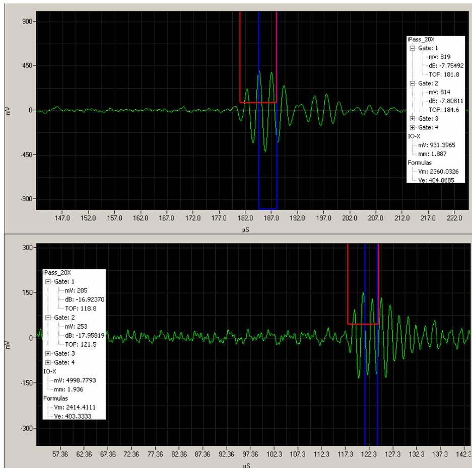
**Fig. 5** Typical signal through the 8-ply 0% porosity CFRP sample: 0.5 MHz (top) and 1.0 MHz (bottom).
