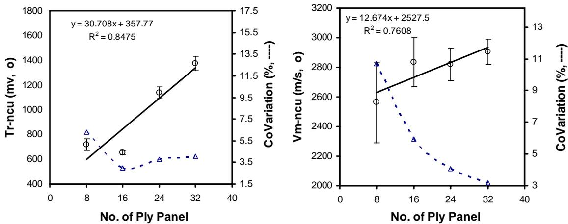
**Fig. 12** Relationship of the transmittance and velocity versus number of plies samples.
