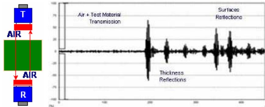
**Fig. 1** Direct transmission schematic diagram and the typical A-scan showing various signals as a function of air and test material. Sample is 50 mm thick polystyrene.
