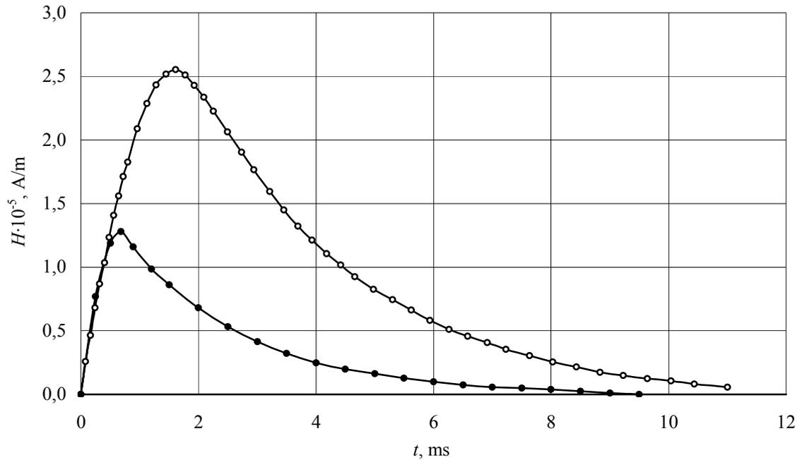
Figure 2. Form of the pulse of normal component of the magnetic field strength on the end face of the transducer of plant IMPOC-1B (○) and plant IMPOC-1BM (●)
