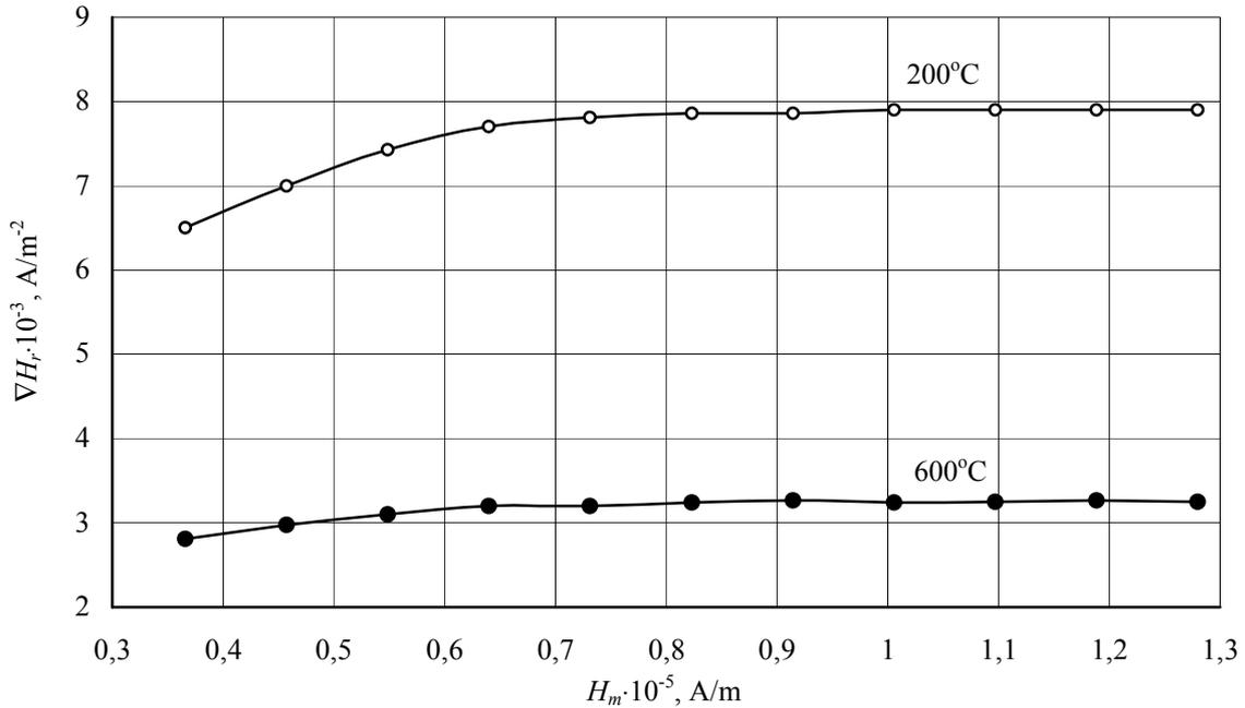
Figure 3. Dependence of indications of the plant IMPOC-1BM on the amplitude of magnetizing pulses for the specimens of steel, containing 0,08 % of carbon, 3 mm in thickness, annealed at temperatures 200 °C and 600 °C.
