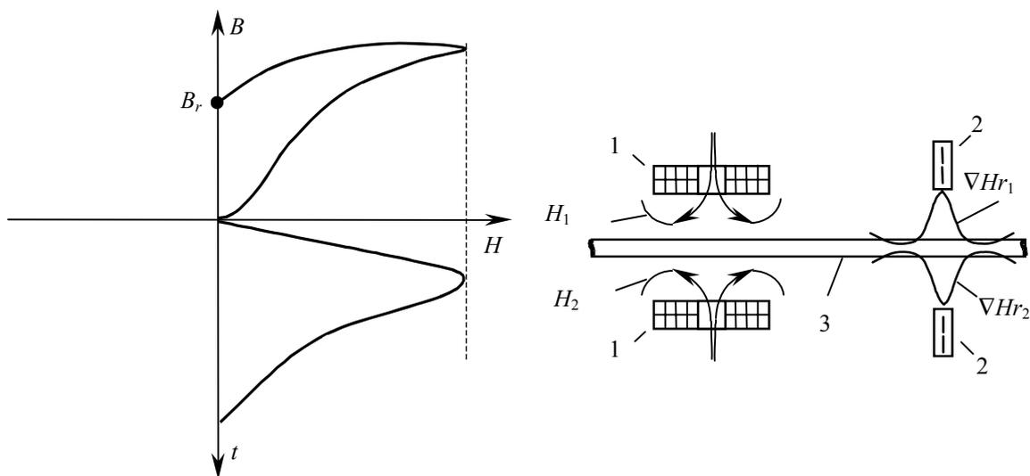
Figure 1. Measuring principle: 1 – magnetizing solenoids; 2 – ferroprobes gradientmeters; 3 – the sheet in motion
