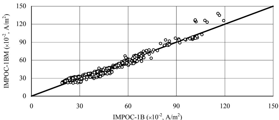
Figure 8. Correlation between the indications of the plants IMPOC-1B and IMPOC-1BM.
