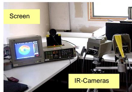
The measurement results will be transferred to a computer and analyzed there. By a gap of 10 cm between the measure point and the object a geometric resolution of ca. 0.5 mm per pixel is yielded.
