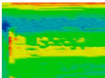
In the PTR figure, the defective heat seal as well as a food product inclusion are quickly and dependably detectable. The sensing of the PTR - signals takes place with more than 100 Hz by a pulse frequency of 50 Hz.
