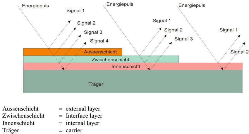
The pulse energy is influenced by each interface and leads to a time delayed process of the energy distribution on the outside of the foil.
