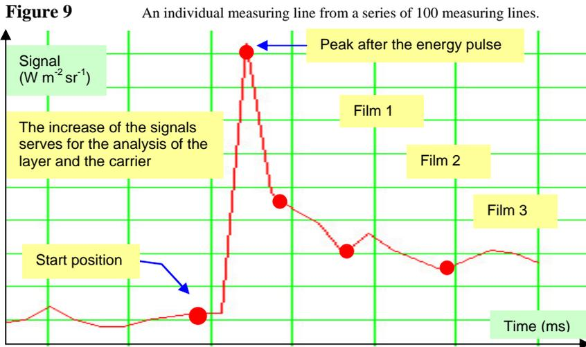
For the measurement, the foil is mounted in front of the measuring head. The space between the measuring head and the foil is between 5 cm and 10 cm. After the energy pulse from the radiances in the function of the spectrum and the time the layer thickness of each individual film can be calculated at the measuring point.
