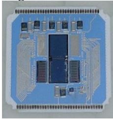
All components on the sensor chip (figure 3) are completely contacted. The operation via the interface to the outside is always guaranteed.
