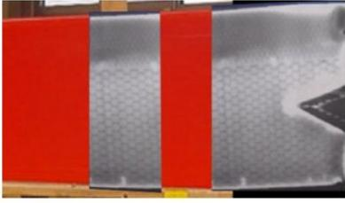
The adhesion of the core in the inside of the wing and the transition between the different honeycomb types can be examined with the speed of 25 cm/s. With the PTR-procedure the layer thickness and variation of the layer thickness can also be determined contact-free, quickly and reliably
