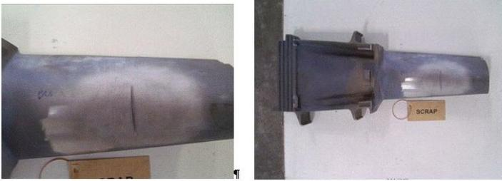
If the crack's depth is larger than 0.75 mm the turbine blade must be replaced. Methods which do not involve destruction tests are used for reliable, accurate and quick determination forof the crack, its direction and depth.
