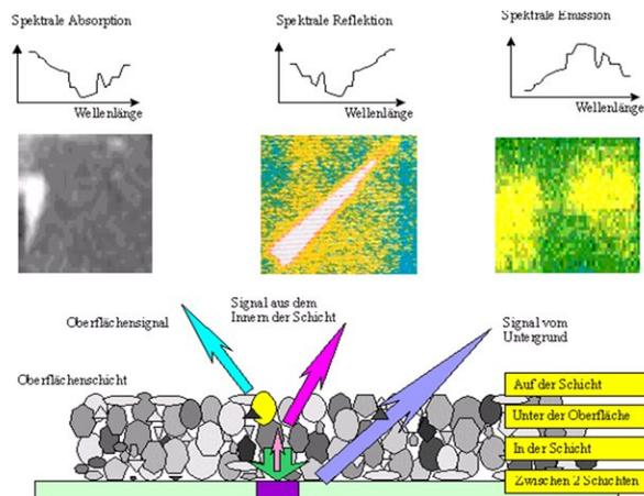
Application and process engineering depend on setting of the tasks and on the material, which should be examined. The information measured at the component surface differs temporally and spectrally, what makes the contact-free defect characterization possible.
