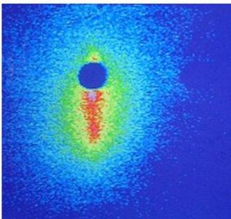
Thermoelastic effect from the impulse with high frequency mechanical oscillations results at the crack's edges. Thus locally increased temperature, dependent on the oscillation and the e-module develops. Temperature registration in the course of the time, synchronized with the oscillation, supplies the data on the type of the crack and its geometry.
