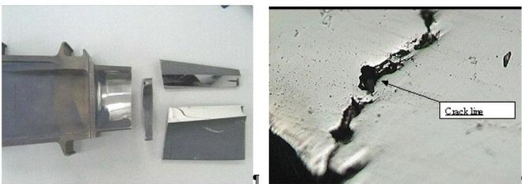
Microscope photograph (picture right) and the cut of the turbine blade (picture left). Often the components are checked with destruction test in order to identify the type of the defect.
