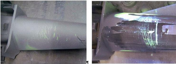
Magnetic particle test at the turbine blade. The finest cracks at the surface can be proven with the procedure. The procedure does not enable a continuous operation.
