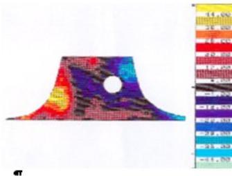
Distribution of the total tension measured with the PTR-procedure at the complicated machine part.
