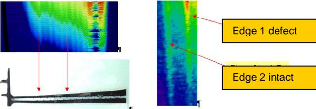
**Adhesion defects and Delamination**
