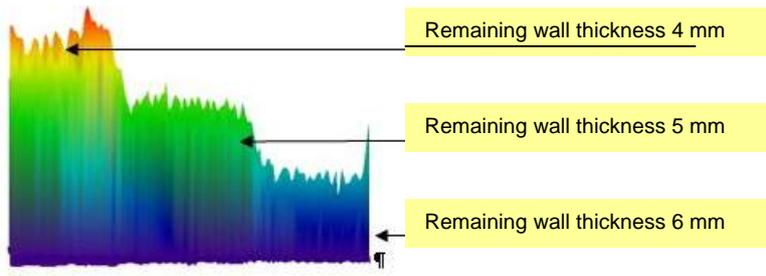
**Determination of the crack's depth**
