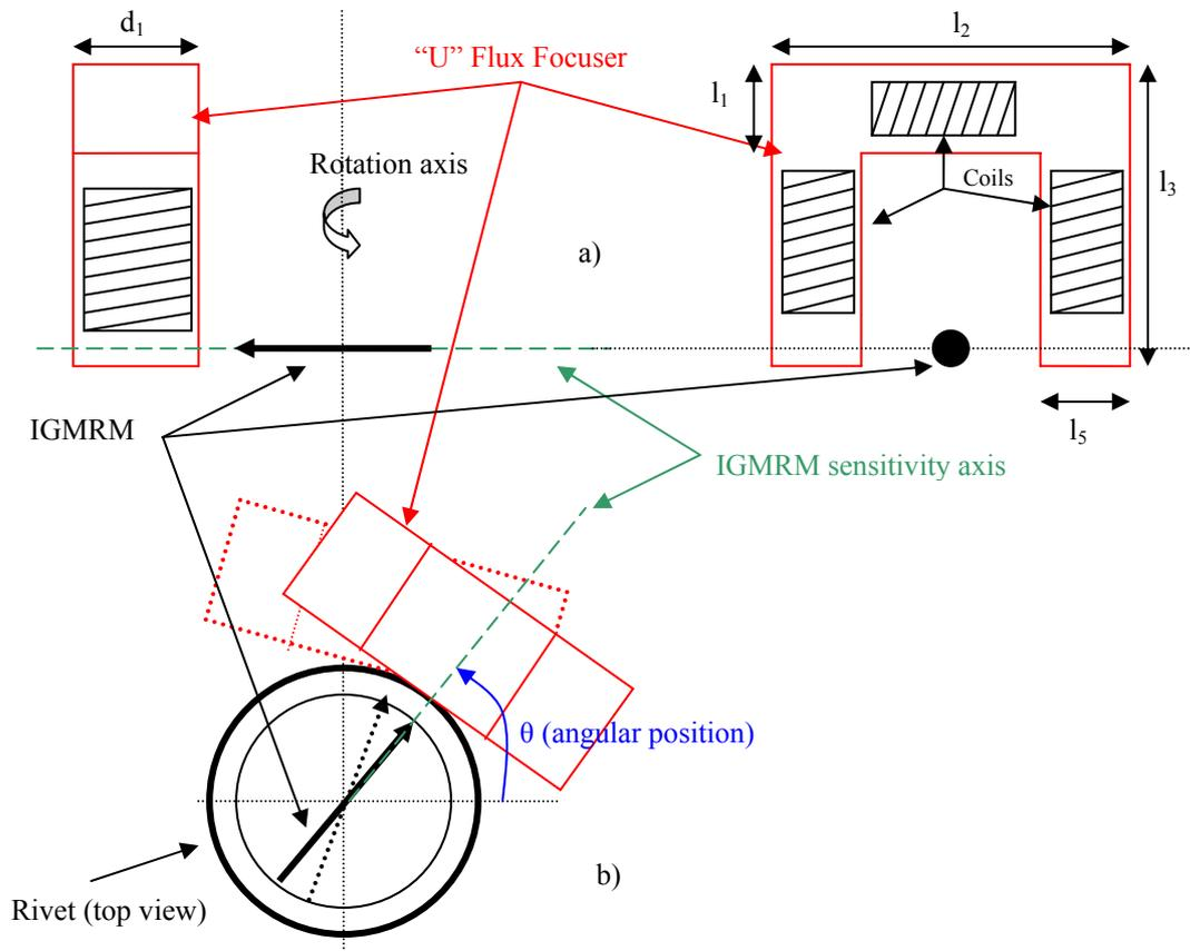
The IGMRM is centered on the axial head rotation. The “U” focuser is placed near the sensing element and is offset to the axial rotation, as given in figure 3.a. Elements are fixed to a rotating support. IGMR sensitivity axis is always directed to the “U” focuser as
