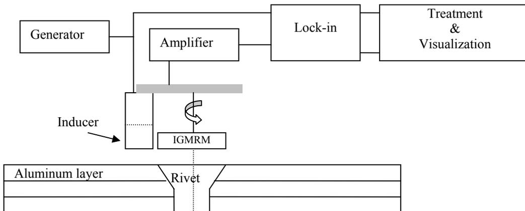
The full eddy current system looks like classical ones. It gives information of the in-phase and out-phase field variations (or amplitude and phase) versus the reference current. A sketch view of the system is presented in figure 1. Its full scale dynamics is around  $120 \text{ dB}/\sqrt{\text{Hz}} + 20 \log(f_0)$  to a maximal value of  $160 \text{ dB}/\sqrt{\text{Hz}}$ , where  $f_0$  is the eddy current frequency [3].
