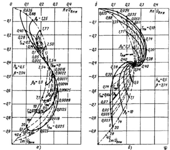
Fig. 2. Hodographs of added voltage of a plane eddy-current probe from surface thickness for various specific conductance
