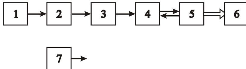
**1 – active oscillator, 2 – plane eddy-current probe, 3 – amplitude detector, 4 – programmable amplifier, 5 – built-in microcontroller, 6 – display, 7 – stabilized power supply block**
