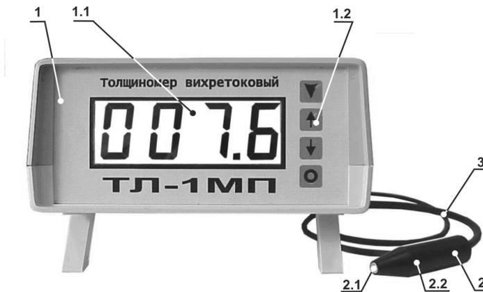
Fig. 4. Galvanic coating thickness gage TL-1MP
