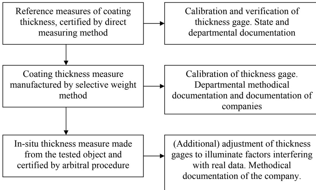
Fig. 5. Metrological provision for galvanic coating thickness inspection
