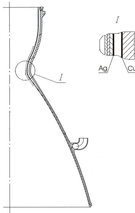
Fig. 1. Section of a combustion chamber body
