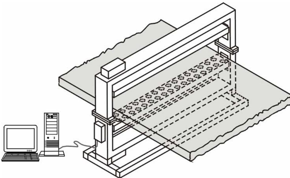
**Fig. 5.** Microwave Process Scanner EM VISION PROCESS
