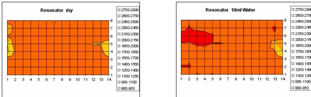
**Fig. 9.** Comparison of Microwave scans without leakage and with small leakage
