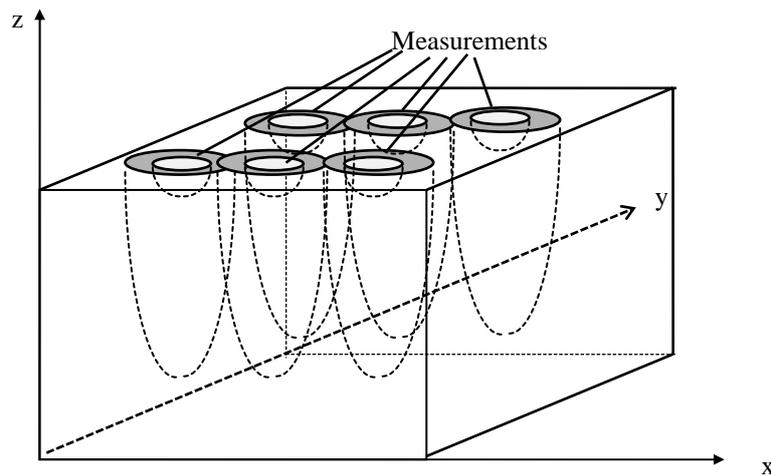
**Fig. 3.** Distribution of measuring volumina with two different microwave applicators
