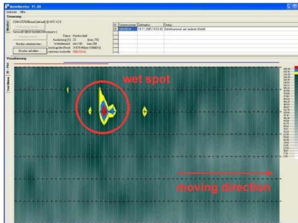
Fig. 8. Microwave online scan of insulating material during production
