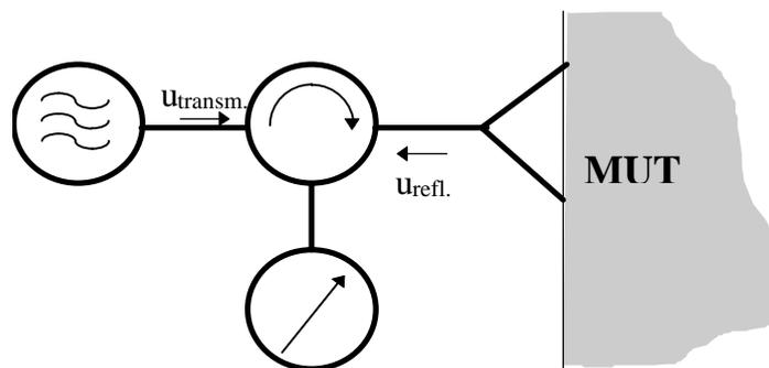
**Fig. 1.** Microwave reflection measurement
