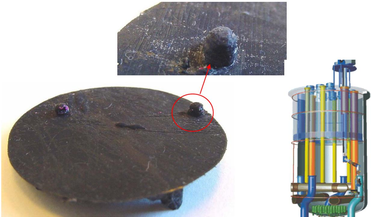
**Figure 3.** Remote application of moulding material through a 6" opening in the reactor vessel head by means of a 6 axis robot developed by FORCE Technology. The left figure shows the result of a wall reduction and the figure to the right shows the robot installed in the reactor vessel.
