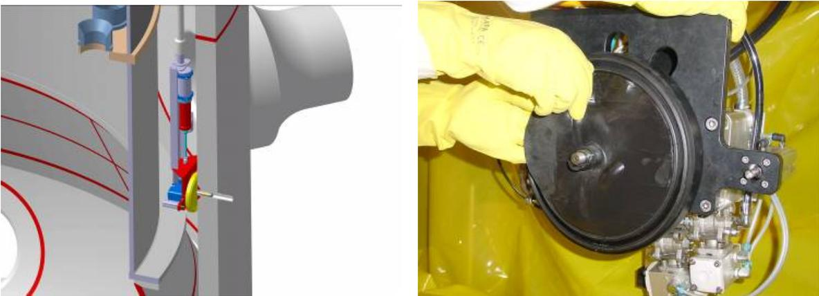
**Figure 4.** The remote application tool is shown fixed in the level measuring nozzle at a water depth of 26 meters. The yellow part forms the outer mould and the component form the inner mould.
