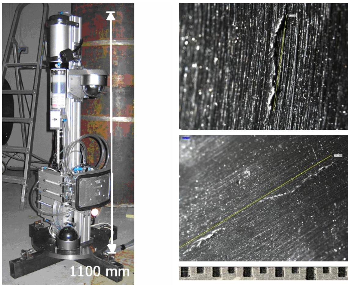
**Figure 6.** The left hand picture shows the remote application tool with surveillance cameras, identification and quality assurance possibilities. The right hand pictures show two microscopic images of two different cracks in an inconel alloy. On the microscopic pictures the surface conditions of the component can be viewed. Below the right hand picture a scale (11 mm) has been included.
