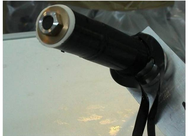
**Figure 5.** The flexible remote application tool mounted on a 2 meter bar for installation into the scram nozzle. Shown to the right, the mould has been made of the scram nozzle.
