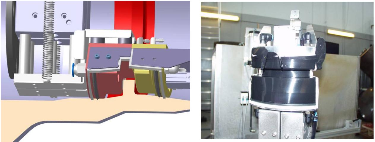
**Figure 7.** The left hand picture shows an advanced two part remote application tool. The remote application tool is equipped with surveillance cameras, identification and quality assurance possibilities. On the right hand picture, the first mould with the advanced moulding tool has been documented.
