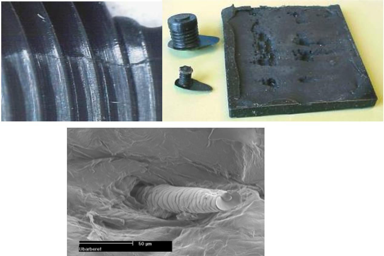
**Figure 2a, b and c.** Upper left hand image shows a crack detected in a thread. The crack is running transverse to the thread. Upper right hand image shows a copy of a heavily corroded surface in a vessel. The lower image is a copy of a human hair after the chin has been shaved for illustration of the resolution capabilities only. The picture is viewed in a modern FIB-SEM.
