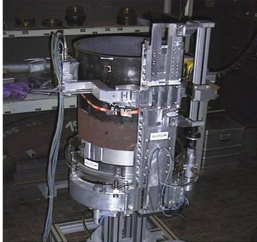
**Fig. 2:** View on one of the first manipulators that was used with the TomoCAR technology.
