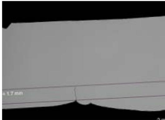
**Fig. 6:** Metallographic view of a stress-corrosion cracking on one of the investigated welds.
