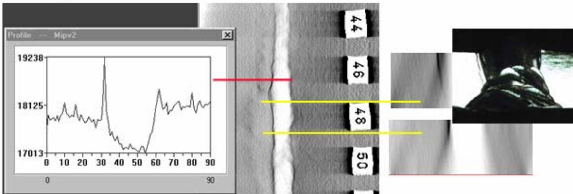
**Fig. 4:** The central part of this image shows the radiograph of one of the studied weld surfaces. The corresponding grey scale profile is on the left part and on the right of the image is the corresponding metallographic image.
