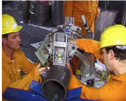
**Fig. 12:** Adjustment of the TomoCAR unit on a client installation.
