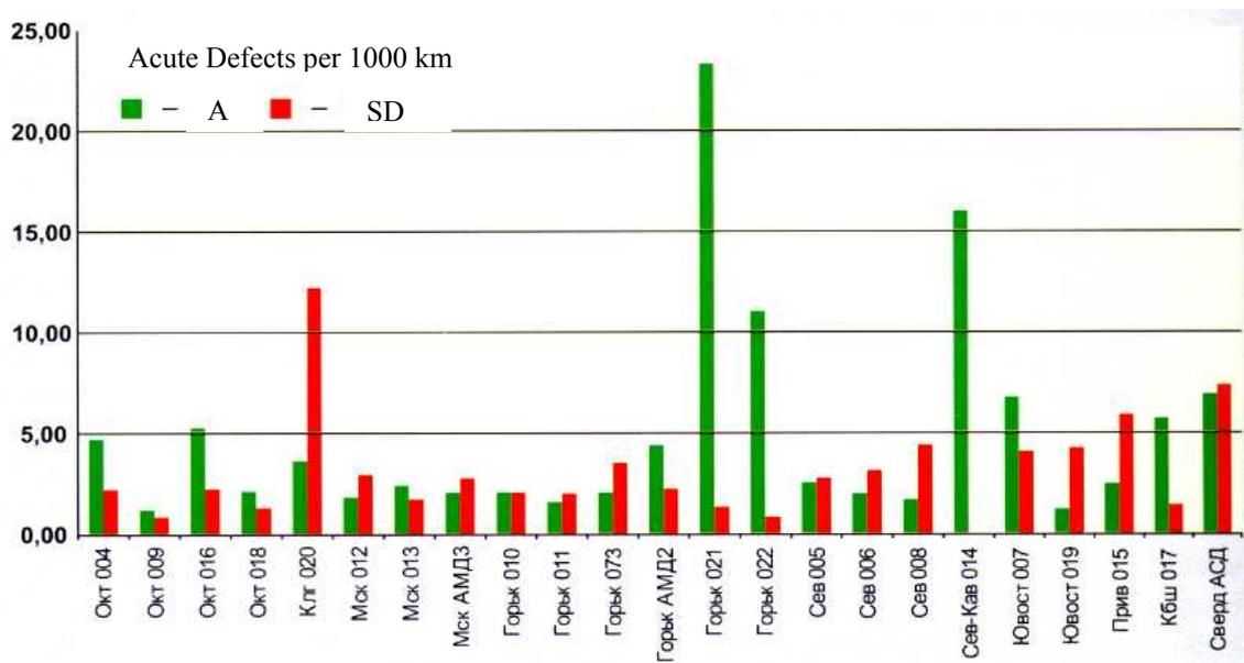
Fig. 5. Detectability of defects in rails with removable defectoscopes and defectoscope road cars in different railroads on the Ministry of Railways network
