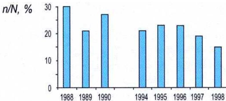
Fig. 4. Ratio of the number (n) of rail breaks because of defects that were not revealed by operators to the total number (N) of breaks per year
