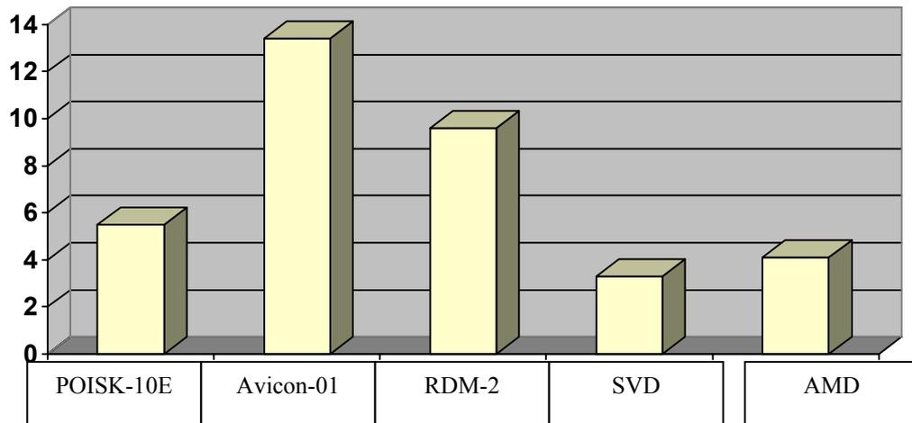
Fig. 7. Actual (year 2003) technical efficiency of continuous nondestructive check means of rails en route (the number of detected defects per 1000 km).
