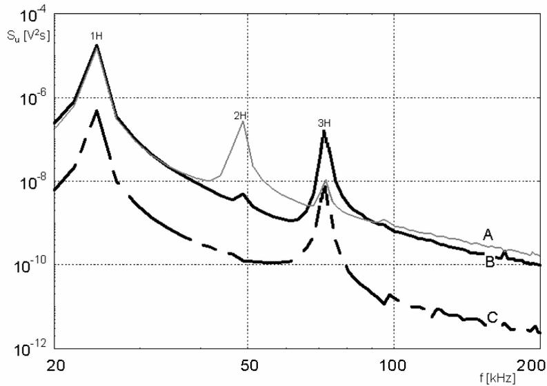
Fig. 4 Response frequency spectrum of ceramic tiles, glazed surface
