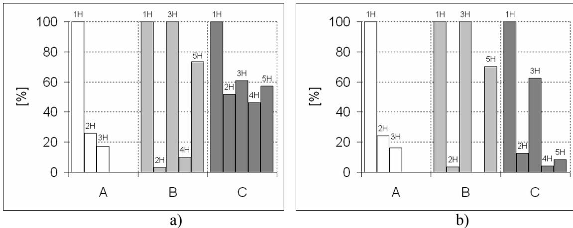
Fig. 7. Frequency spectra of specimen response - normalized amplitude magnitudes, a) exciting on the glazed surface, b) exciting on the non-glazed surface
