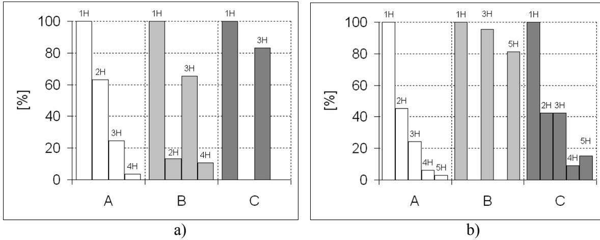
Fig. 6. Frequency spectra of specimen response - normalized amplitude magnitudes, a) measuring and exciting on the glazed surface, b) measuring and exciting on the non-glazed surface
