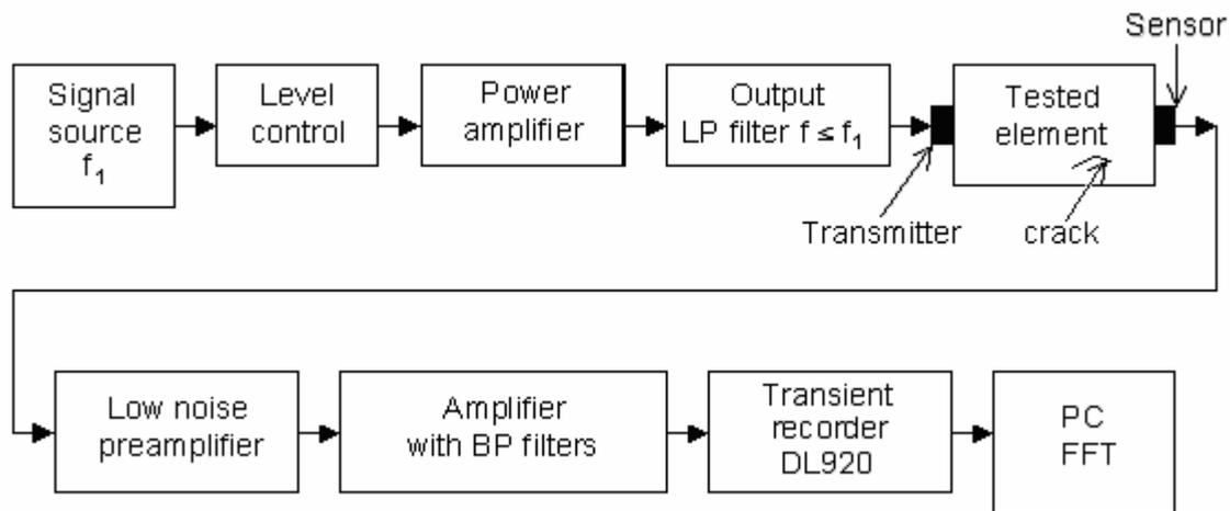
Fig. 1 Block scheme of the measure equipment
