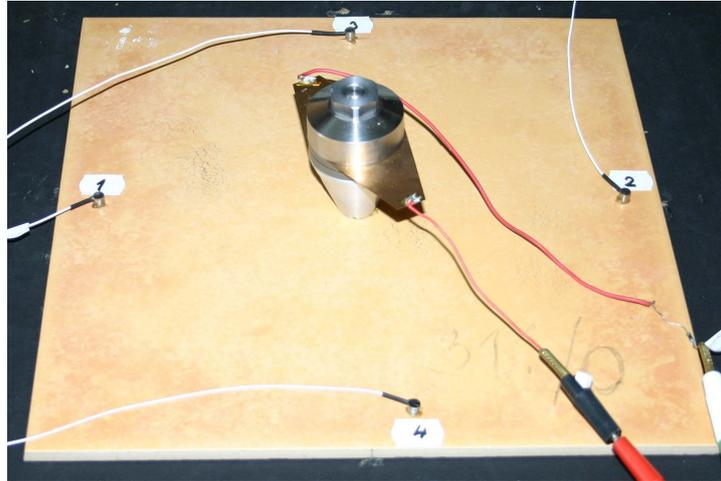
Fig. 2 Test specimen with transmitter and sensors
