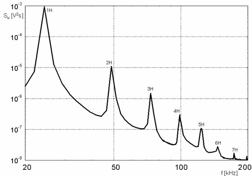
Fig. 3 Response frequency spectrum of duralumin sheet
