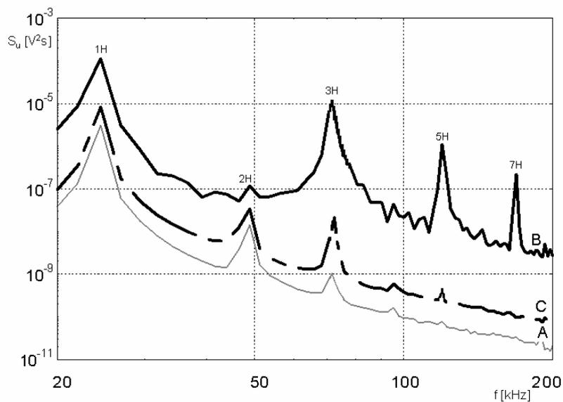
Fig. 5 Response frequency spectrum of ceramic tiles, non-glazed surface
