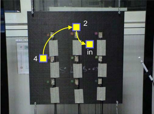
Figure 8: Impact tests locations
