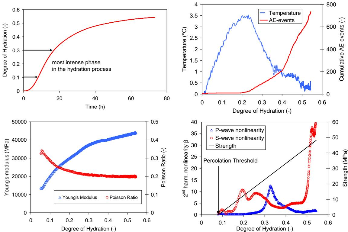
Figure 3: Evolution of the degree of hydration with time, and parametric representation of the variation in internal temperature, cumulative AE events, Young's Modulus and Poisson Ratio, and nonlinear elastic coefficients in DYNA 0.33 as function of the degree of hydration.
