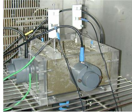
Figure 1: Cell used for monitoring the hardening process in young concrete, containing two pairs of compressional (P) and shear (S) transducers, two Acoustic Emission (AE) sensors and two temperature (T) sensors.
