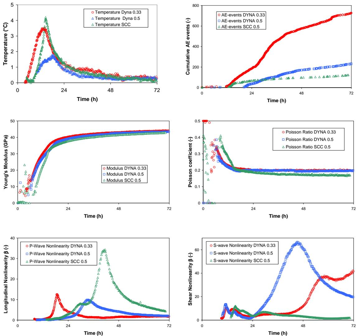
Figure 4: Comparison of the evolutions of the internal change in temperature, the cumulative AE events, the Young's Modulus and the Poisson Ratio, and the P and S wave nonlinearity in DYNA 0.5, DYNA 0.33 en SCC 0.5 during the first 3 days of the curing process.
