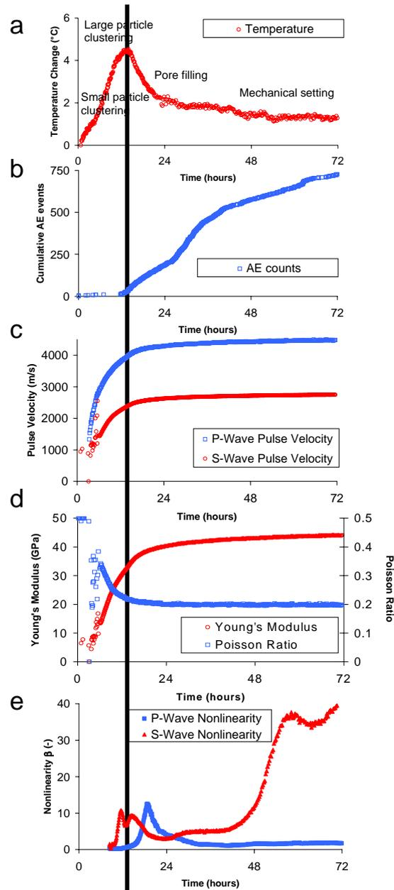
Figure 2: Typical monitoring results for the hydration process of DYNA 0.33 during the first 3 days: From top to bottom: evolution of temperature, cumulative AE events, P and S wave velocities, Young's Modulus and Poisson Ratio, and P and S nonlinear elasticity.
