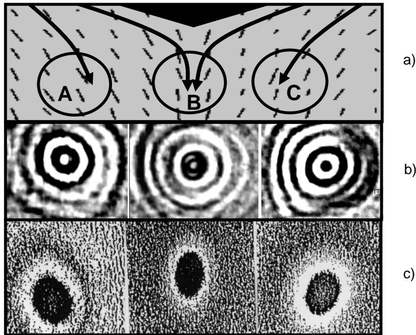
Figure 5. Measurements of local fibre anisotropy in short glass fibre reinforced composites.
