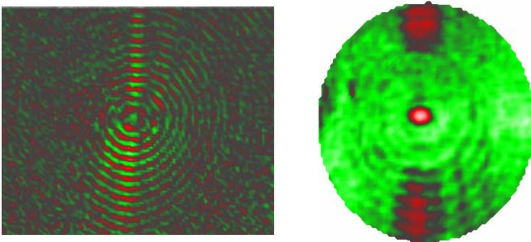
Figure 7. Phonon-focusing of air-coupled flexural wave in a single-component composite: view over the scanning area 35x30 mm (linear scale, left); zoomed image in dB-scale (right).
