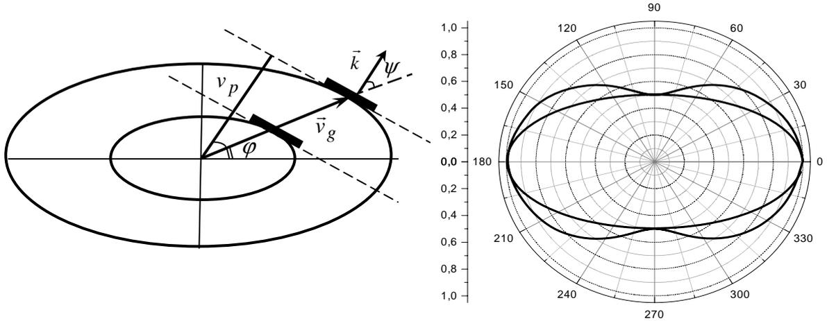
Figure 2. Energy flow and phase velocity in wavefront pattern (left); reconstruction of phase velocity pattern from elliptical wavefront (right).
