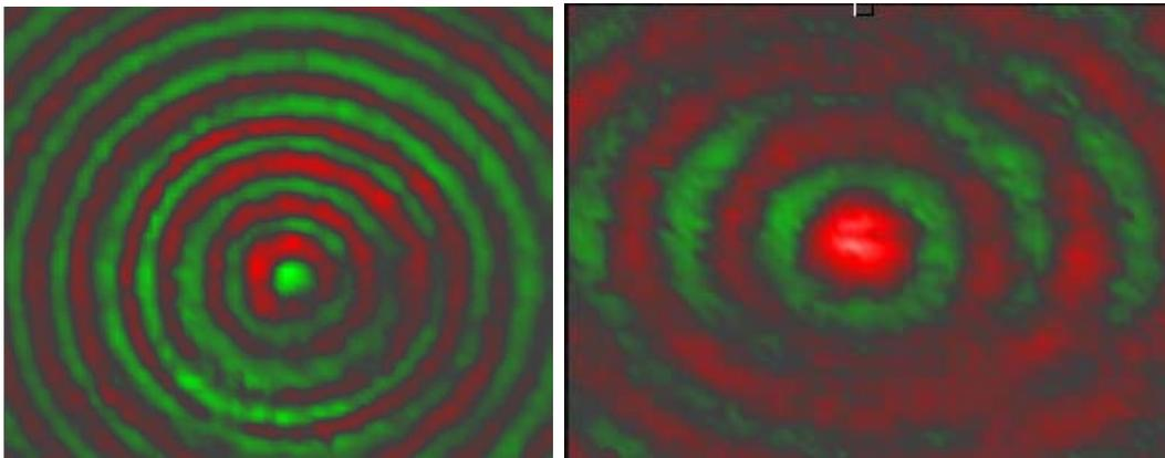
Figure 4. Wavefront patterns for SAW in PMMA (left) and flexural wave in CFRP (right).
