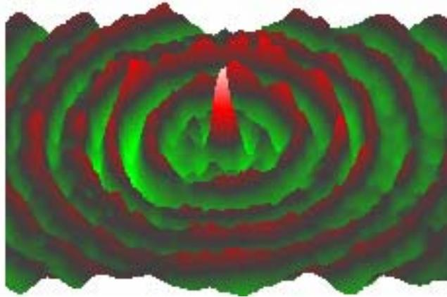
Figure 3. Wave field excited by focused air-coupled transducer in 1.2mm plate of polycarbonate.
