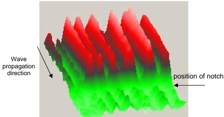
Figure 6. Phonon focusing due to waveguide effect in annual rings of wood.
