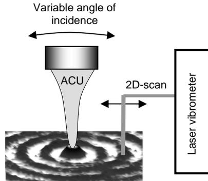
Figure 1. Layout of air-coupled phonon-focusing.
