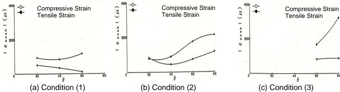
Fig. 9. Strain peak versus ply angle
