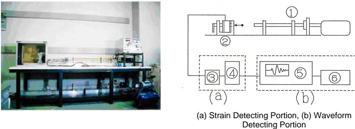
**Fig. 2.** Schematic diagram of an air-gun type of impact apparatus
