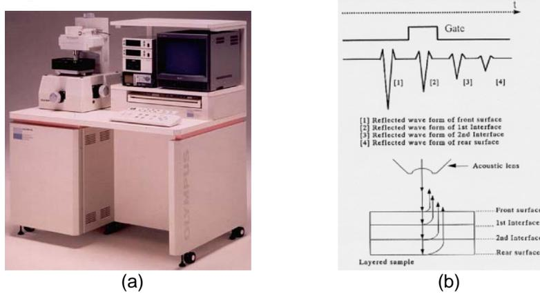
**Fig. 5.** (a) A schematic diagram of a mechanical scanning acoustic reflection microscope (SAM; pulse-wave mode). The SAM operates with frequencies ranging from 5MHz to 250MHz. (b) Ultrasonic waves reflected from the specimen. The “gate (*i.e.*, rectangular electrical signal)” was multiplied to the signal reflected from the interface B to visualize a horizontal cross-sectional acoustic image (C-scan Image) at the interface A.
