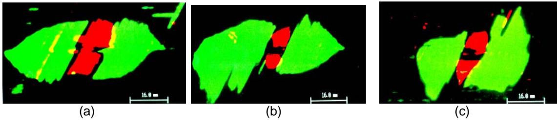
**Fig. 6.** Acoustic images show delaminations at interfaces A and B of the specimen C60, wherein the delaminations were introduced by the steel ball impact. The images were formed by the acoustic lens for pulse wave mode with the frequency at 30MHz. (a): Delaminations introduced without loading, (b): Delaminations introduced under compressive loading, (c): Delaminations introduced under tensile loading.
