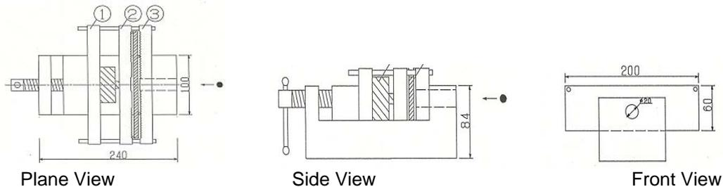
**Fig. 3.** Schematic diagram of the unsymmetrical 4-Points Bending Apparatus
