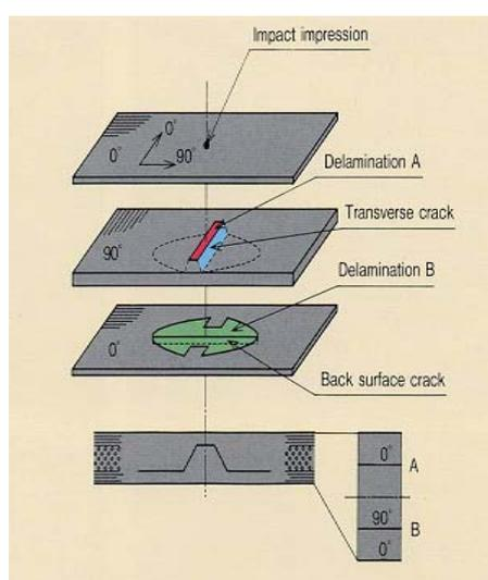
**Fig. 1.** Schematic diagram of CFRP structure for the specimen denoted as C90. The delaminations at interfaces A and B are named “Delamination A” and “Delamination B.”
