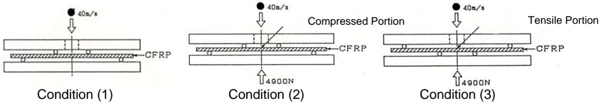
**Fig. 4.** Condition (1): Impact the steel ball (diameter: 10mm; velocity: 40m/s; air pressure:  $4.9 \times 10^4$  Pa) onto the surface of the CFRP without loading. Condition (2): Impact the steel ball onto the surface including compressed portion with loading (4900N). Condition (3): Impact the steel ball onto the surface including tensile portion with loading (4900N).
