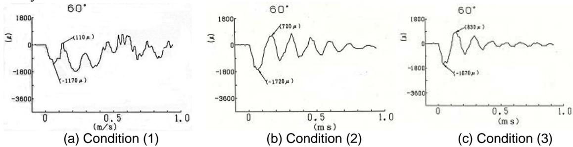
Fig.8. Strain change of rear surface at impact
