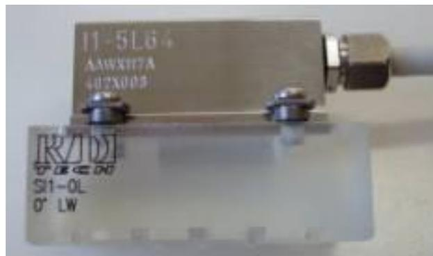
Fig. 12: 64 Element array on plexi delay line
