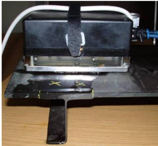
Fig. 28: Steering beam, excited by different time delays
