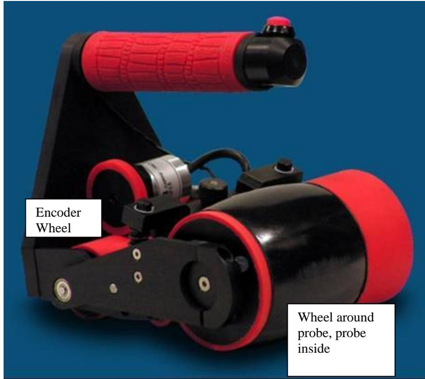
Fig. 20: Wheel Probe, NDT Solutions
