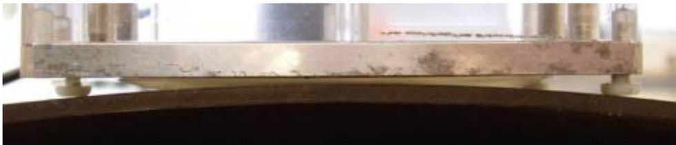
Fig. 18: Waterbox stable via contact points on a curved aircraft structure
