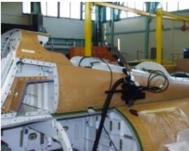
Fig. 8: X/Y Scanner on Flexi Track
