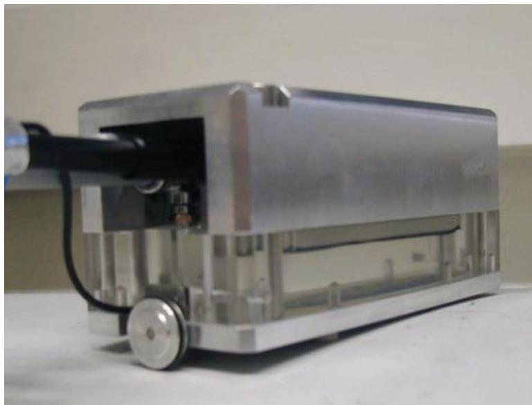
Fig. 19: Water Box with Integrated small Encoder
