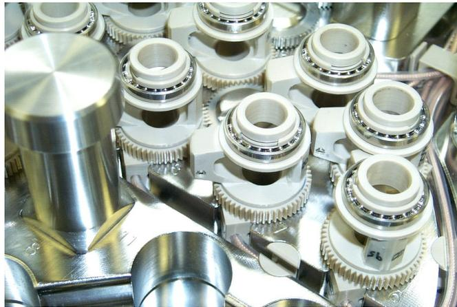
Figure 2: Detail of the UT probe rotation system
