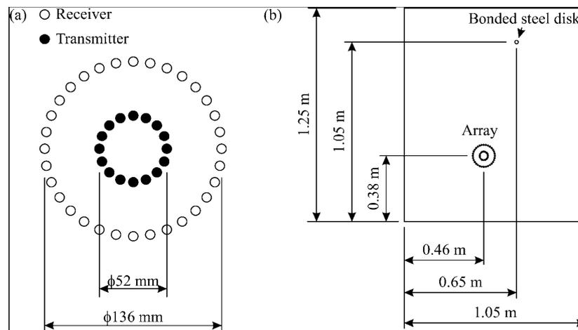
Fig.4. a) Geometry of EMAT array;
