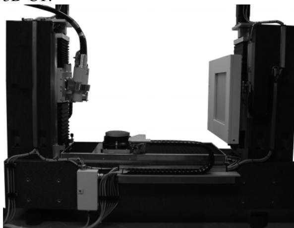
Fig. 3 CT-System (high precision manipulator, 400 mm x 400 mm detector array, “mini-focus” XRay system)
