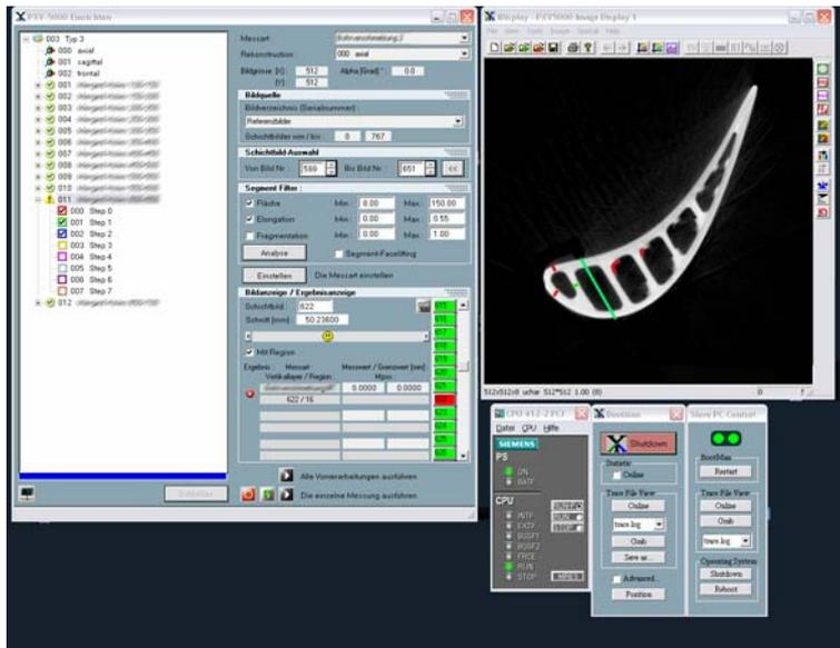
Fig.2 Automatic evaluation of structural and geometrical object features with PXV5000
