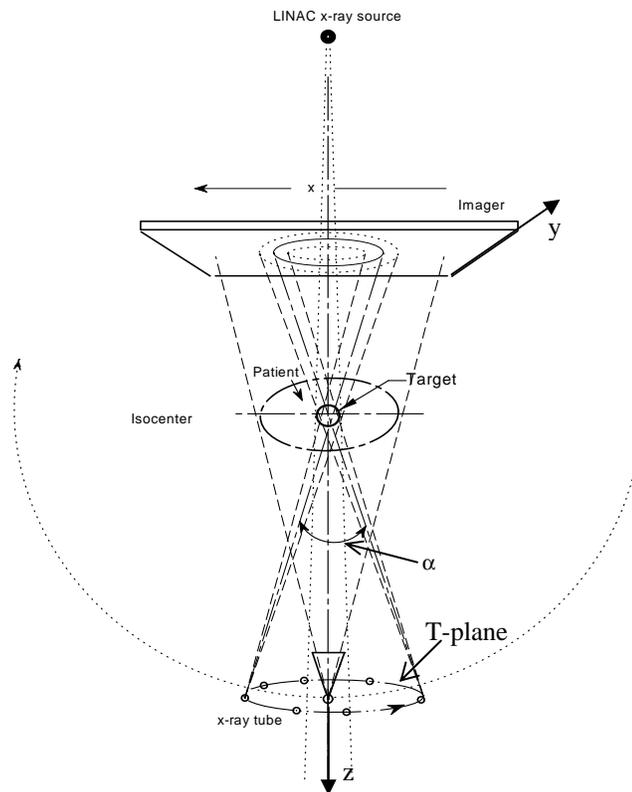
Fig. 2. Data acquisition geometry outline. Trajectory of an X-ray tube is parallel to the detector plane,  $\alpha$  - solid angle.
