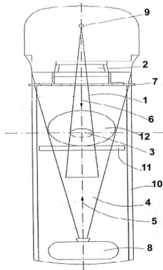
Fig.1.Chart of the combined Radiation Therapy&Diadnostic Setup: 1-therapy beam; 2-Multi Leaf Collimator; 3-ROI with tumor; 4-kV beam; 5- main Setup axle; 6-therapy beam direction; 7-2D imager; 8-kV X-ray tube; 9-MEV photon target; 10-gantry; 11-couch; 12-patient.
