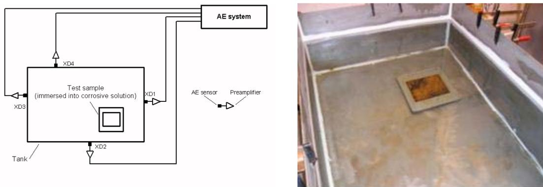
**Figure 2:** Sketch of lab test set-up (left) and plate of ship building steel immersed in corrosive liquid (right)
