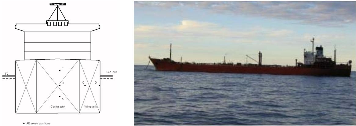
**Figure 3:** Sketch of mid ship section (left) of tanker 'Icarus II' (right)
