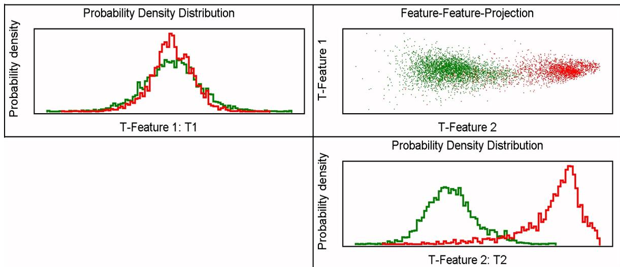
**Figure 4:** Separation of corrosion and background AE signals in the feature space (Visual Class<sup>TM</sup>)
