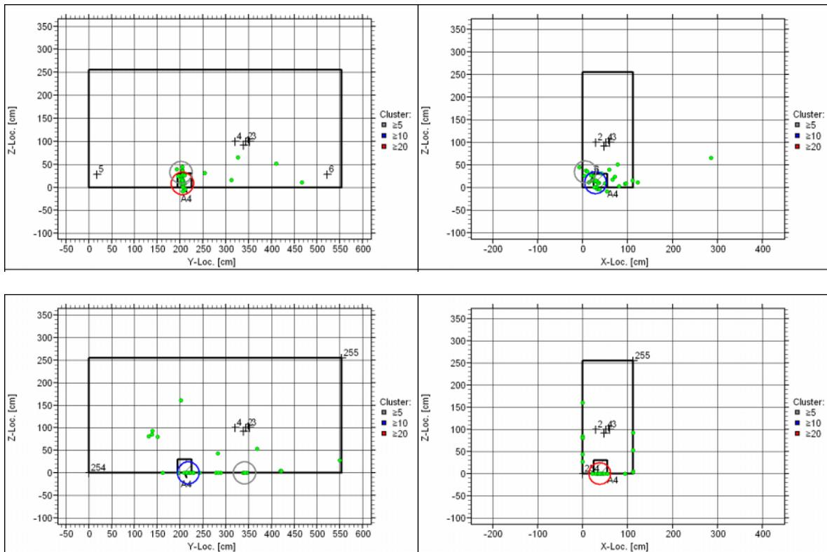
**Figure 5:** Comparison of source location obtained by 3d location algorithm used for permanent installation (top) and by the MUSA location algorithm (bottom) used for spot testing.
