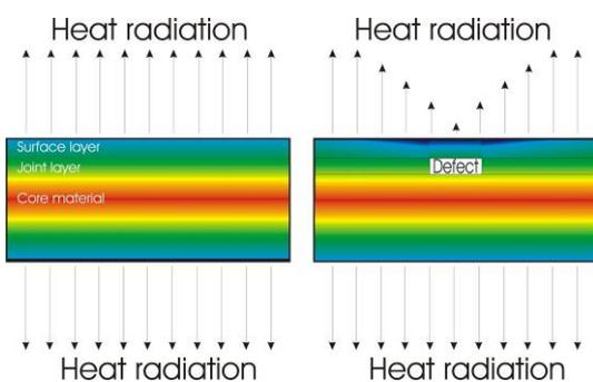
Fig. 2: Principle of the passive online thermography.
