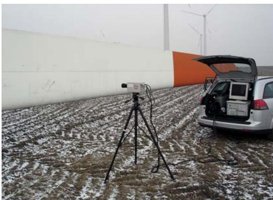
Fig. 8: Photo of the IR-camera during the passive inspection of the blade.
