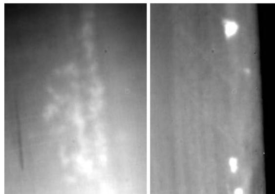
Fig. 18: Thermal images taken from the measurement shown in Fig. 17. Clearly visible are delaminations in the blade (left) and air bubbles in the trailing edge (right).
