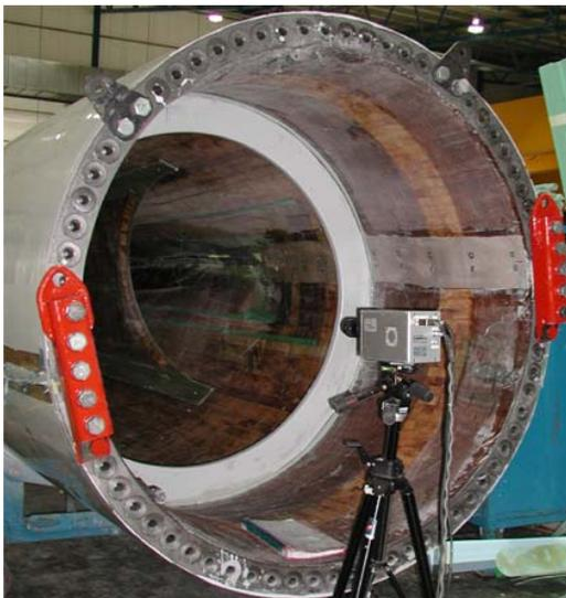
Fig. 4: Photo showing the passive inspection of the inner part of the rotor blade with an IR-camera.
