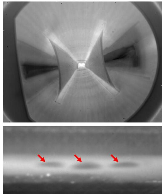
Fig. 5: Thermal image of the rotor blade from inside (top) and defect gluing indexed by red arrows on the leading edge (bottom) observed from outside.
