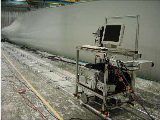
Fig. 11: Active online thermography setup on a trail for the inspection of long structures.
