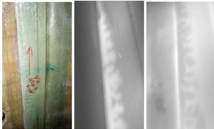
Fig. 16 Photo of a glue joint (left) and thermal images showing the defects (air gaps) in reflection mode (centre) as hot spots or in transmission as cold spots (right).
