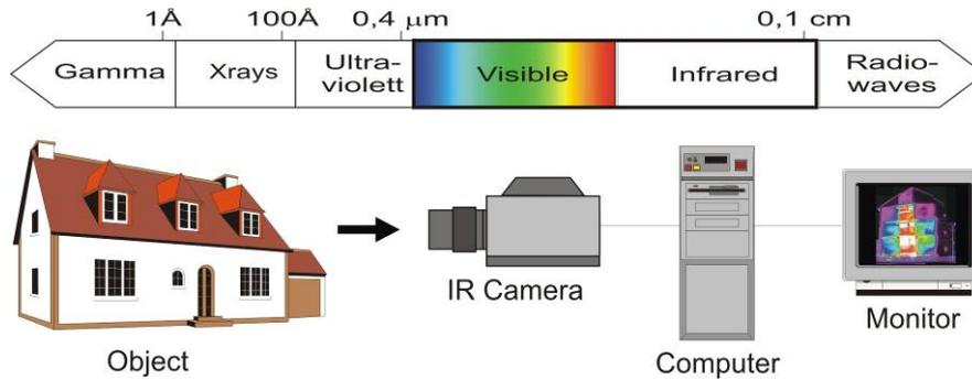
Fig. 1: Image processing setup using an IR-camera to visualize even small temperature differences on the objects surface.
