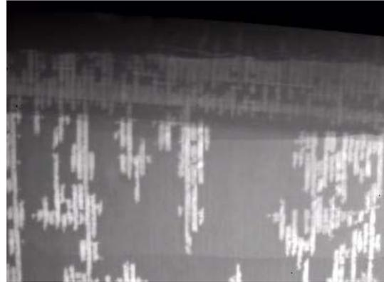
Fig. 12: Extended air bubble inclusions can be detected with online thermography.
