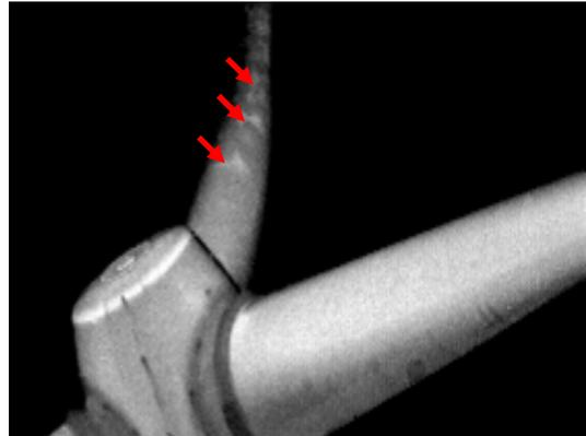
Fig. 7: Thermal image of the rotor while it is moving. The bright areas indicate delaminations produced by heat due to the friction of micro cracks.
