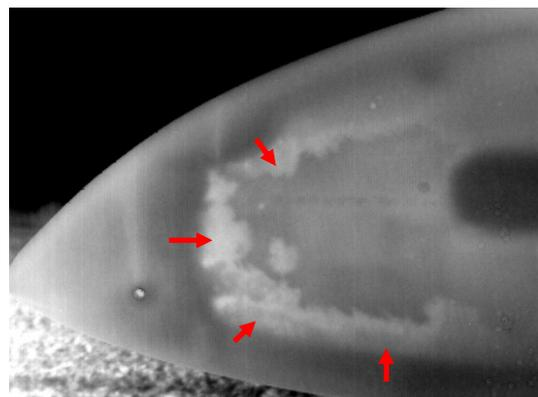
Fig. 9: Long time after sunset, the thermal image of the tip of the rotor blade is showing the frozen water (arrows) inside the blade.
