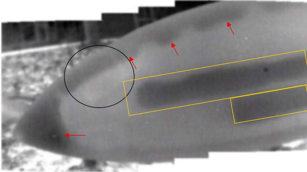
Fig. 10: Thermal image of the rotor blade showing important structures like the gluing at the trailing edge (arrows), the twin main spars (rectangular) and a repaired area (circle).
