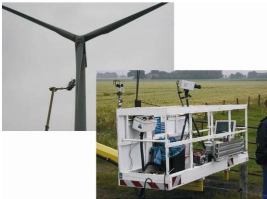
Fig. 17: The measurement system fixed at the working platform of the lift (right) and working in a height of about 100 m (left).
