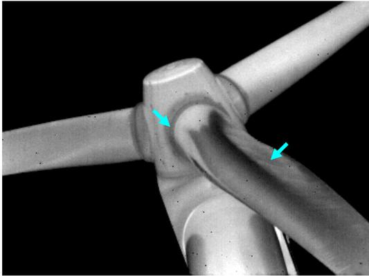
Fig. 6: Thermal image of the rotor while it is moving. The bright areas are warmer as the dark areas and show the heat production due to mechanical loading (blue arrows).
