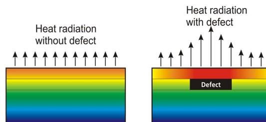
Fig. 3: Principle of the active online thermography.
