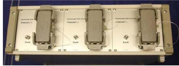
**Fig. 12:** HISO1 rear view with 3 Q-CON-F quadruple coaxial-connectors and earthing points
