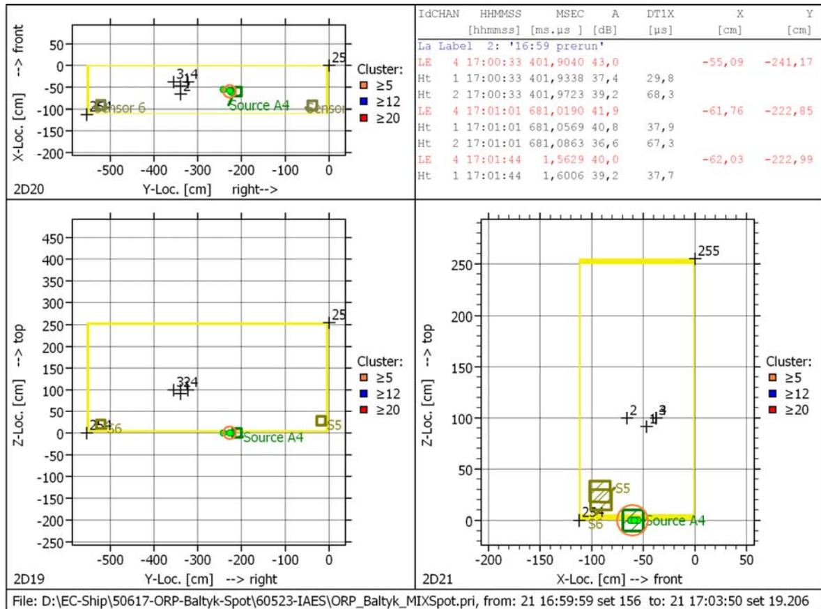
**Fig. 8:** “Cuboid” Location algorithm determines location on the bottom or on a surrounding wall.
