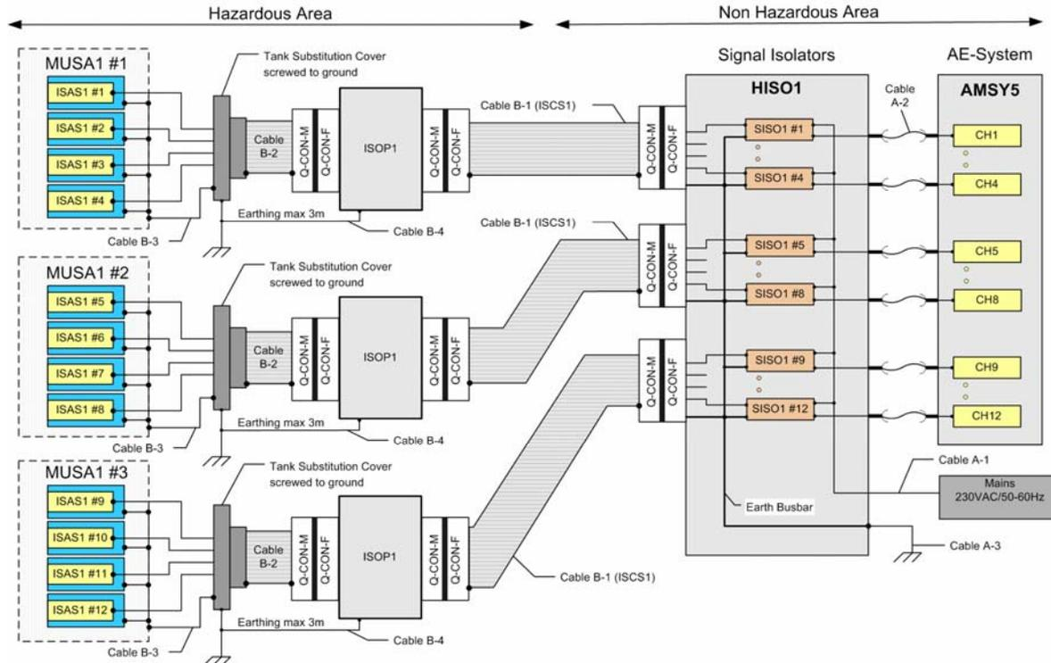
**Fig 1:** Block diagram of product family ISAFE with connection to the AE-system (AMS5-5)
