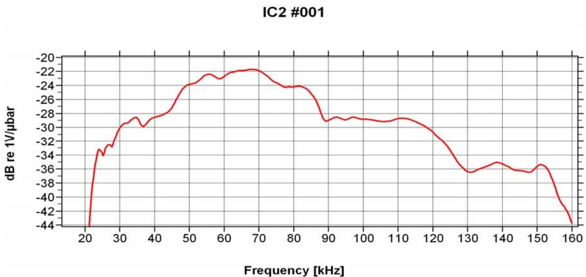
**Fig. 3:** Frequency response of ISAS1 at 40dB gain
