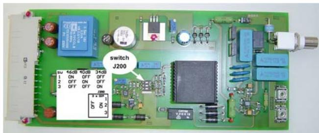
**Fig. 10:** Signal isolator SISO1
