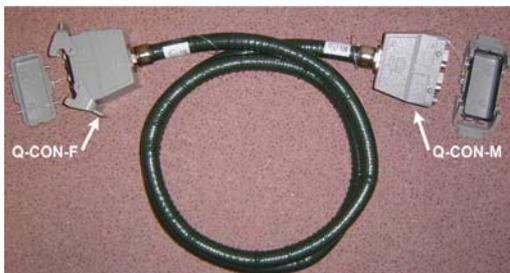
**Fig. 9:** Cable set ISCSI (2m) with quadruple coaxial connectors Q-CON-F and -M
