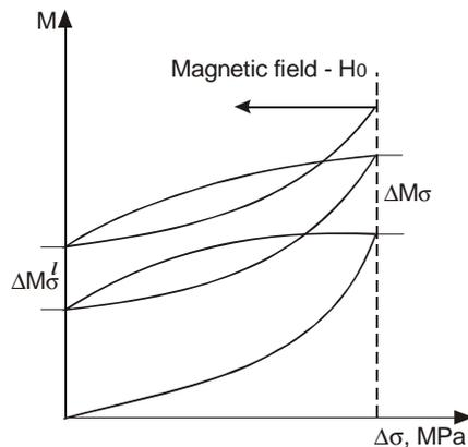
**Figure 1.** The diagram of magneto-elastic effect action:  $\Delta M_\sigma$  and  $\Delta M_\sigma^H$  – change of residual magnetization, accordingly, under loading and after unloading;  $\Delta\sigma$  – change of cyclic loading;  $H_0$  – external magnetic field.
