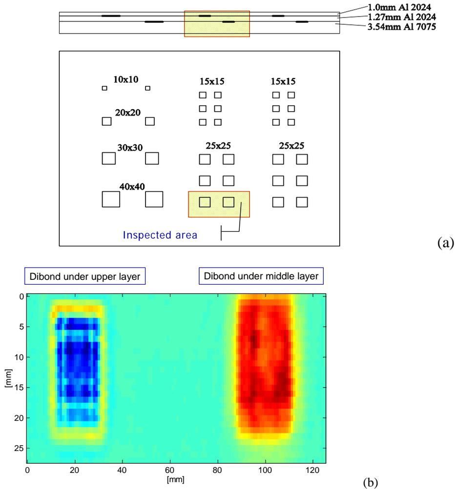
**Figure 6.** Results of NBUS inspection of the specimen Wing Skin with artificial disbonds. Specimen structure (top) and the NBUS scan of the indicated area with two disbonds (bottom).
