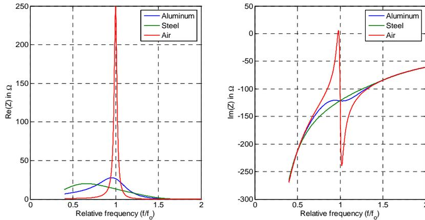
**Figure 3.** Impedance of an example 1 MHz transducer close to its  $f_0$  in the air (red), after loading it with aluminum (blue) and steel (green).
