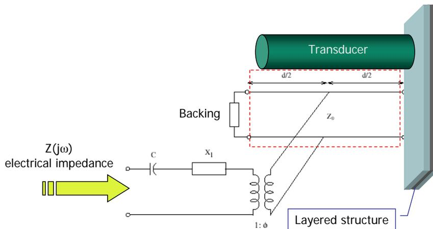
**Figure 1.** Principle of the narrow band resonance inspection of a layered structure.
