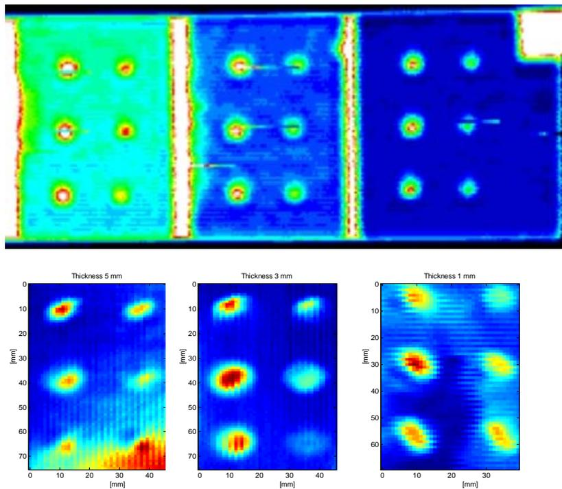
**Figure 8.** Inspection results obtained for the step-wise specimen of CFRP. Ordinary ultrasonic C-scan obtained in through transmission (upper panel) and C-scans obtained using the NBUS from one side (lower panels).
