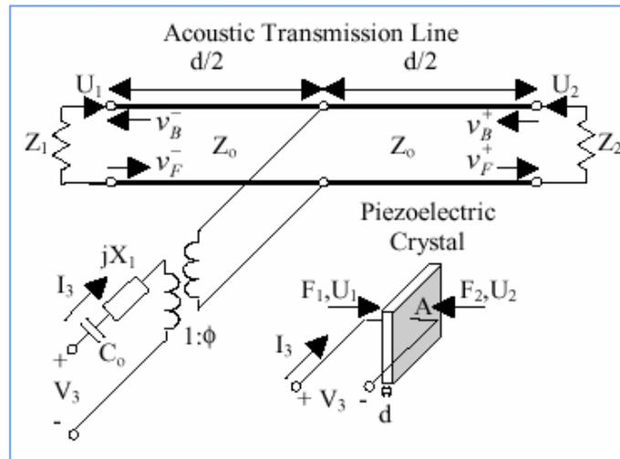
**Figure 2.** The KLM model of a piezoelectric transducer in thickness mode.
