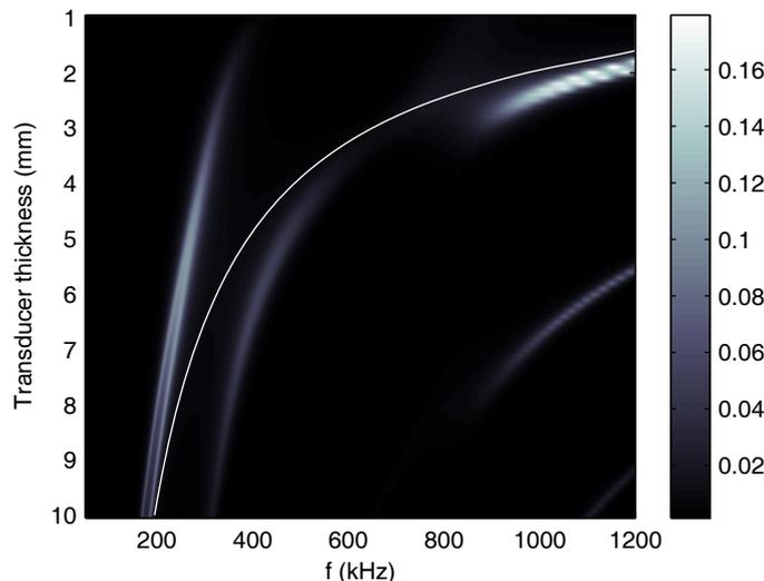
Figure 4. Relative admittance change of a +1µm thickness change in the water coupling layer (the nominal coupling thickness is 30µm). White solid line indicates resonance frequency of the free oscillating transducer in air.
