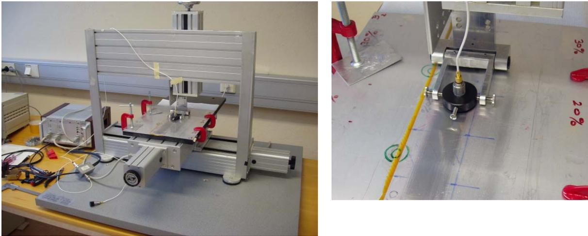
**Figure 5.** The scanning system used in experiments (left), and a detail of transducer suspension (right).
