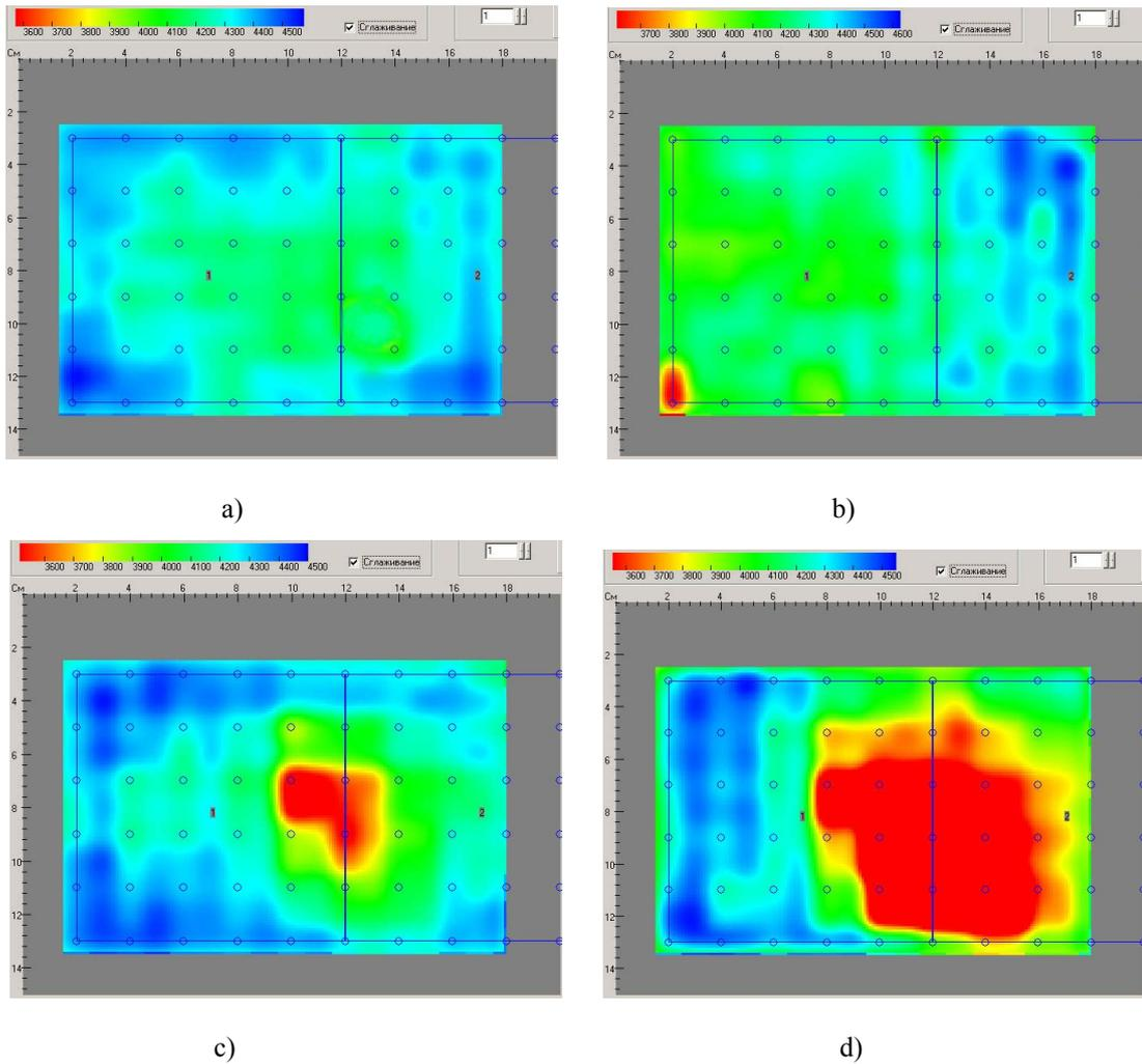
Fig. 3. a) non-defected block; b) block with a defect 20x20 mm; c) block with a defect 40x40 mm; d) block with a defect 60x60 mm.
