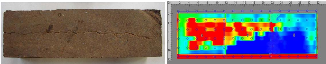
Fig. 4. Photo of block with crack and software processed image.
