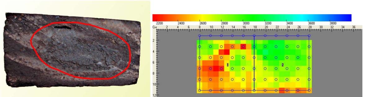
Fig. 6. Photo of block with underburning and software processed image.
