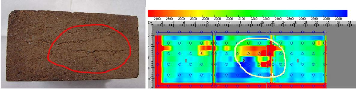
Fig. 5. Photos of block with crack and software processed image.
