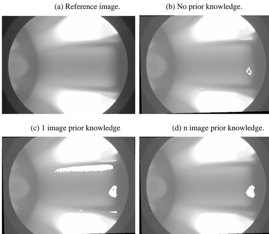
**Figure 3.** Defect recognition using variable prior knowledge.
