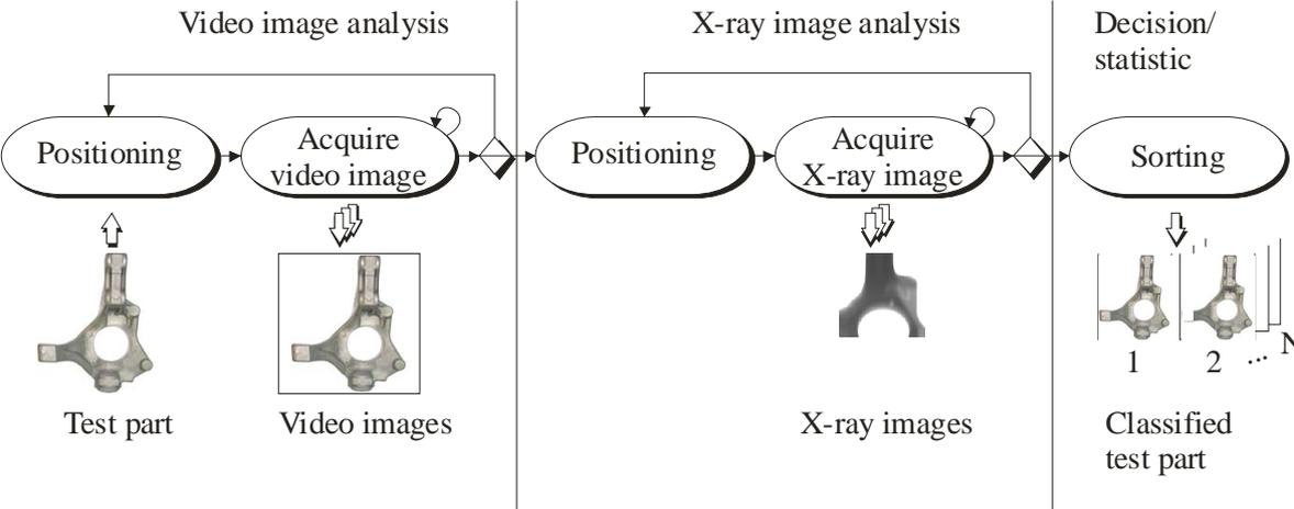
**Figure 1.** General X-ray testing process
