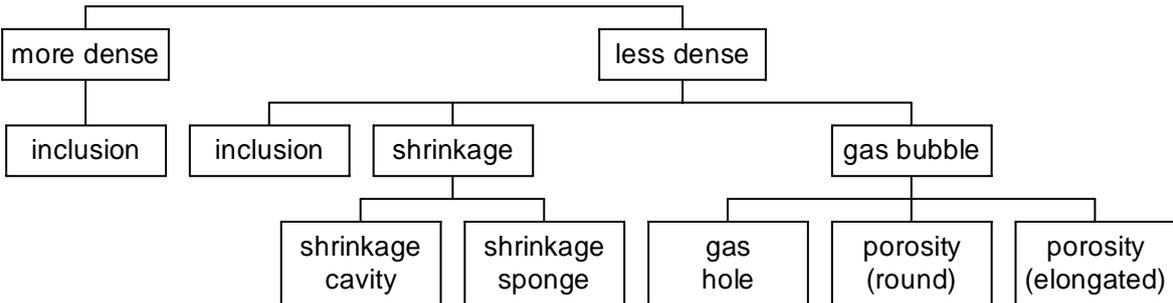
**Figure 2.** Decision tree of detailed classification pursuant to ASTM E2422 (cp. ASTM E155).
