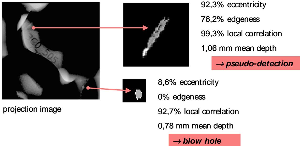
Figure 6: Two examples of faults, the upper one is identified as a false-positive detection, the lower one is a true fault.
