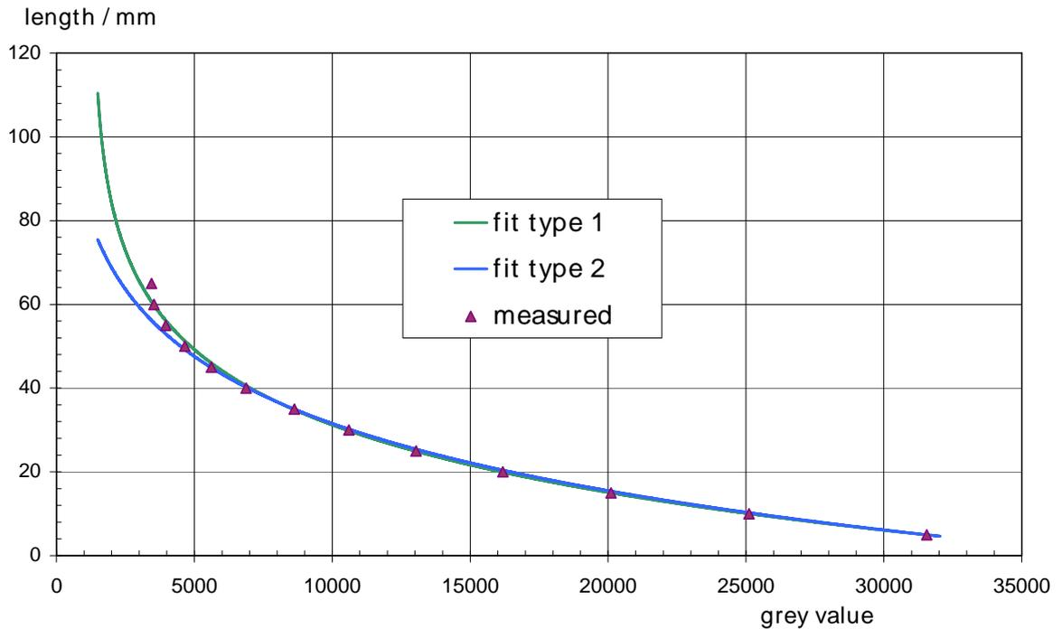
Figure 2: Grey value calibration curves with different fit functions based on the measurements (triangles) with a aluminium step wedge.
