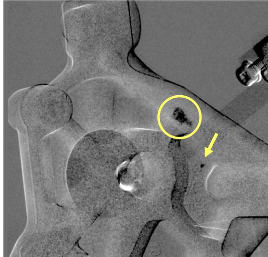
Figure 5: A typical subtraction image from the current and the fault-free reference. A large defect is indicated by the circle, a small defect by an arrow.
