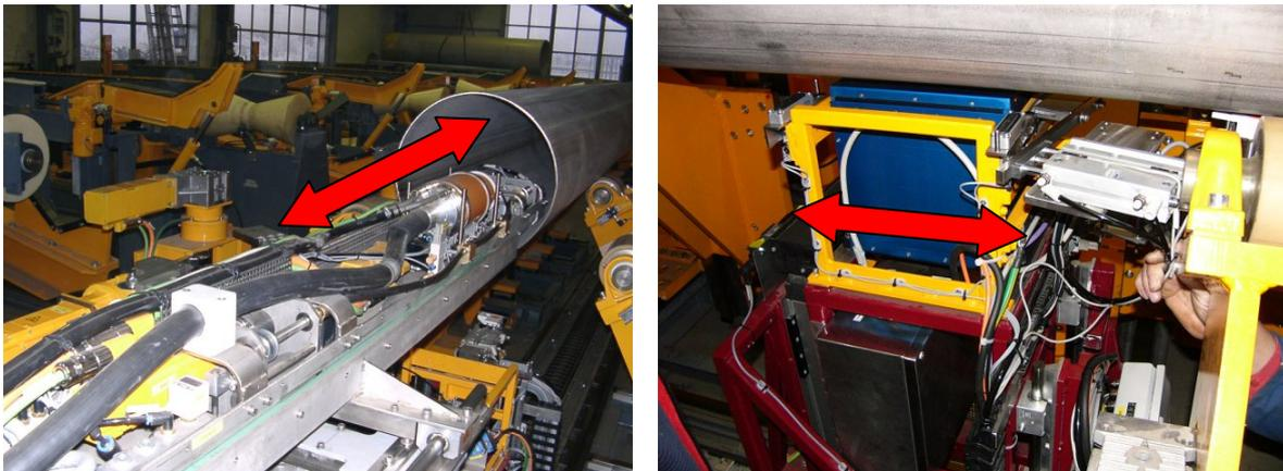
Fig. 3: Carriage and frame with X-ray source and detector (moving directions indicated)
