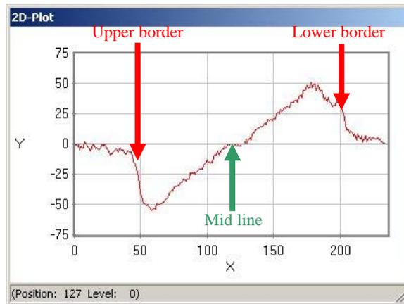
Fig. 7: Gradient of the cross section and detected borders
