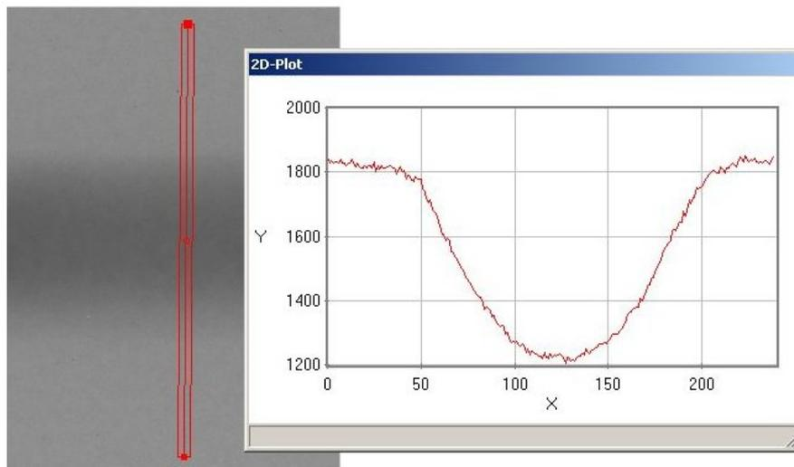
Fig. 6: Cross section of x-ray image of a welded seam and corresponding profile
