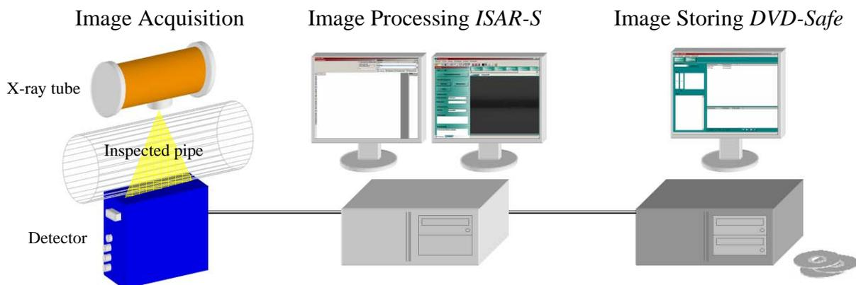
Fig. 1: Integration of system components
