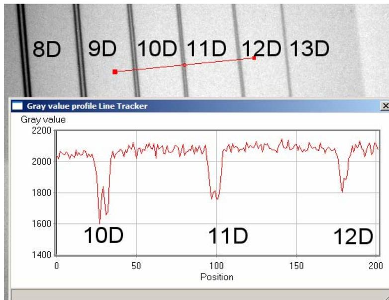
Fig. 5: Double wire test according to EN 462-5 and line profile
