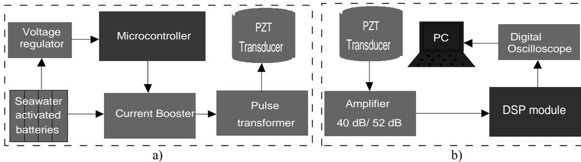
**Figure 1.** Underwater ultrasound system showing their instrumentation main components; a) transmitter and b) receiver.
