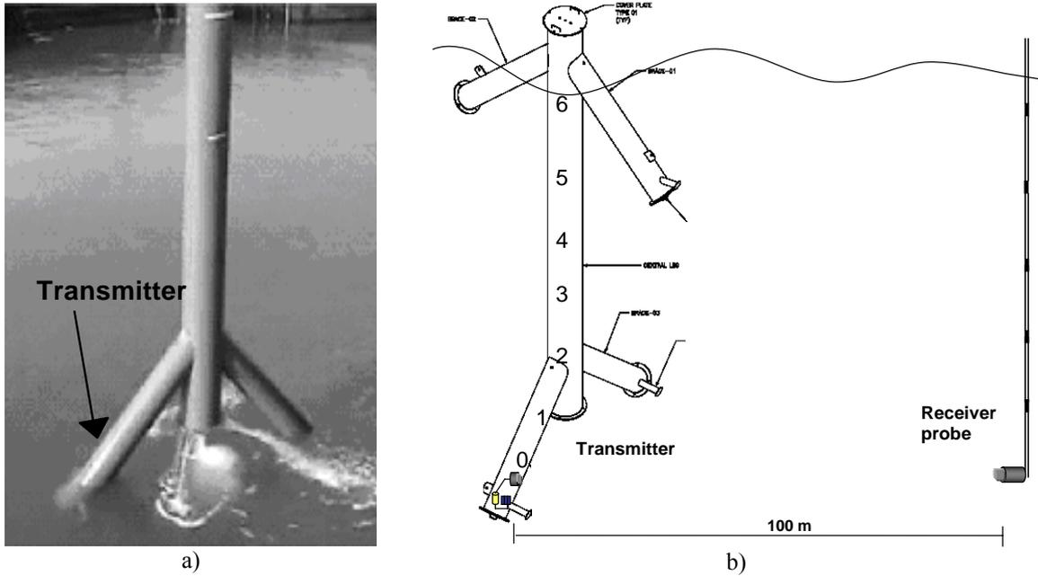
**Figure 3.** Experimental setup using a jointed steel pipe structure, 7m x 0.5m x 16mm; a) being immersed in seawater; b) receiver and transmitter transducers separation.
