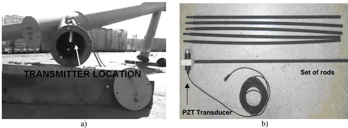
**Figure 2.** a) Transmitter location; b) receiving transducer and a set of rods
