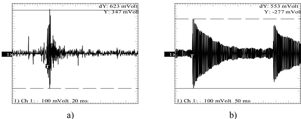
**Figure 4.** Typical signals detected in the underwater ultrasound FMD system using a 34 kHz – 42 kHz chirp, with the structure immersed to a depth of 6 m; a) original received signal at 40 m and an amplitude of  $3.09 \mu\text{V}$ , processed by an FIR filter; (b) original received signal at 100 m and an amplitude of 650 nV, processed by an IIR filter.
