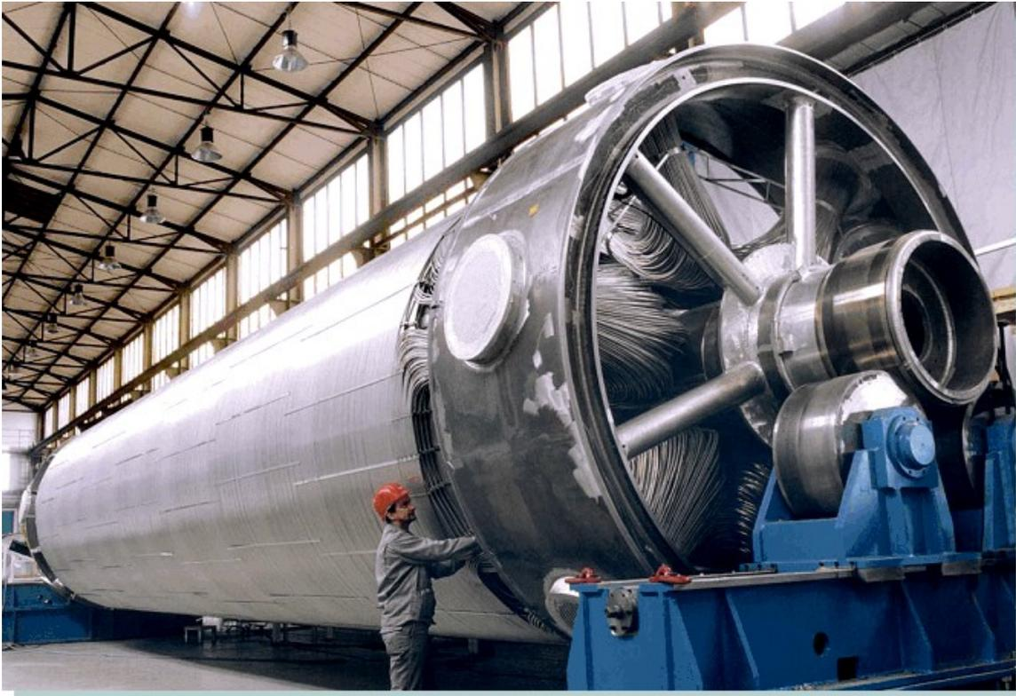
Figure 3: Typical spiral-wound heat exchanger for LNG plants
