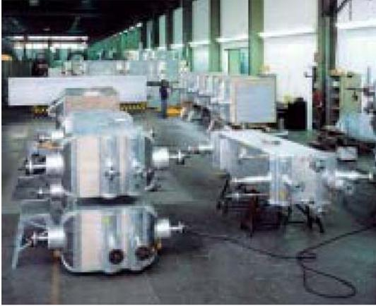
Figure 1: Typical plate-fin heat exchangers for LNG plants
