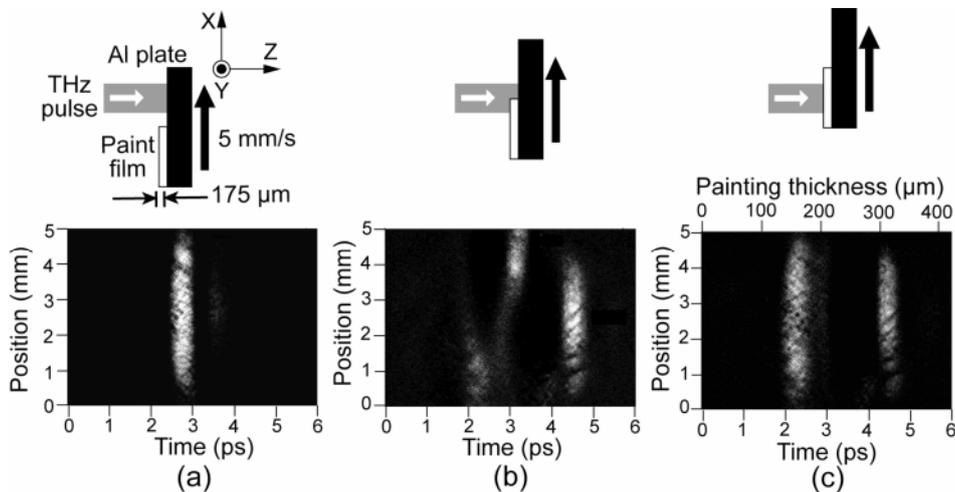
Fig. 3. 2D THz tomography at three different illuminating positions of the moving half-paint film (image size = 6 ps  $\times$  5 mm). (a) Unpainted area, (b) boundary between unpainted and painted areas, and (c) painted area.
