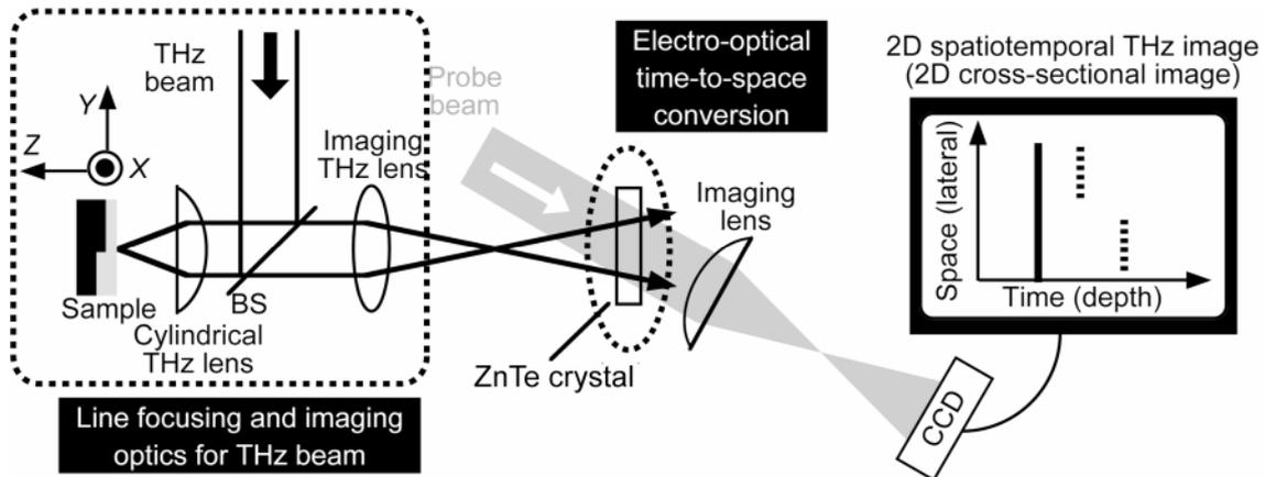
Fig. 1. Experimental setup of real-time 2D THz tomography. CCD: charge-coupled-device camera; BS: beam splitter.
