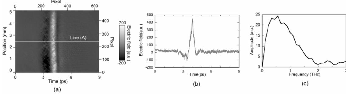
Fig. 2. 2D spatiotemporal THz image of a plane Al mirror surface (image size = 9 ps  $\times$  5 mm). (a) CCD image for an exposure time of 70 ms. (b) Temporal waveform of the THz electric field extracted from a line profile of the 2D spatiotemporal THz image and (c) corresponding spectrum of THz amplitude.
