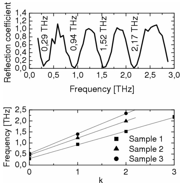
**Figure 3.** Top: Measured reflectivity of an anti-reflection-coated silicon wafer. Bottom: frequency of the observed reflection minima vs. order number k for three samples. The lines indicate linear fits.
