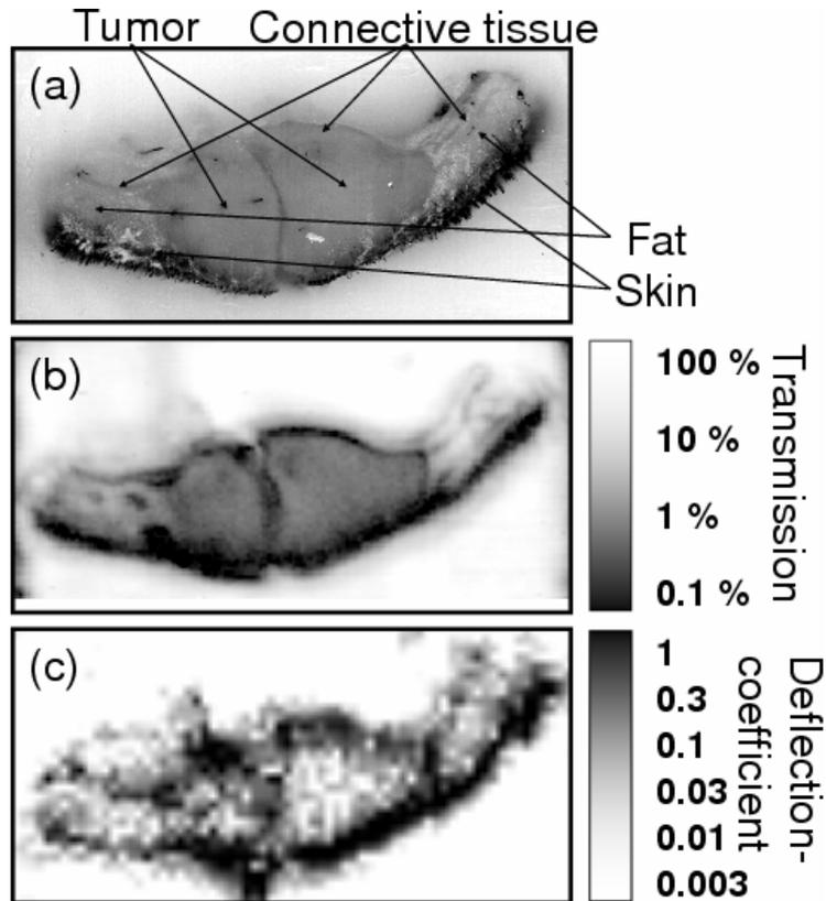
**Figure 1.** (a) Photograph of an archived tissue sample of a cut through a canine skin tumor. (b) Cw transmission image of the sample at 1 THz.(c) Deflection coefficient at 2 THz obtained with a pulsed dark-field system
