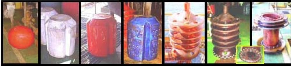
Figure 1 – Cleaning Pigs used in the cleaning operation
