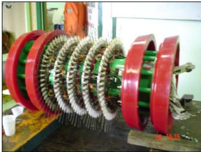
Figure 5 – Feeler Pig assembled for inspection, provided with 250 sensors, two hodometers. The electronic unit and the batteries are housed inside the pig.
