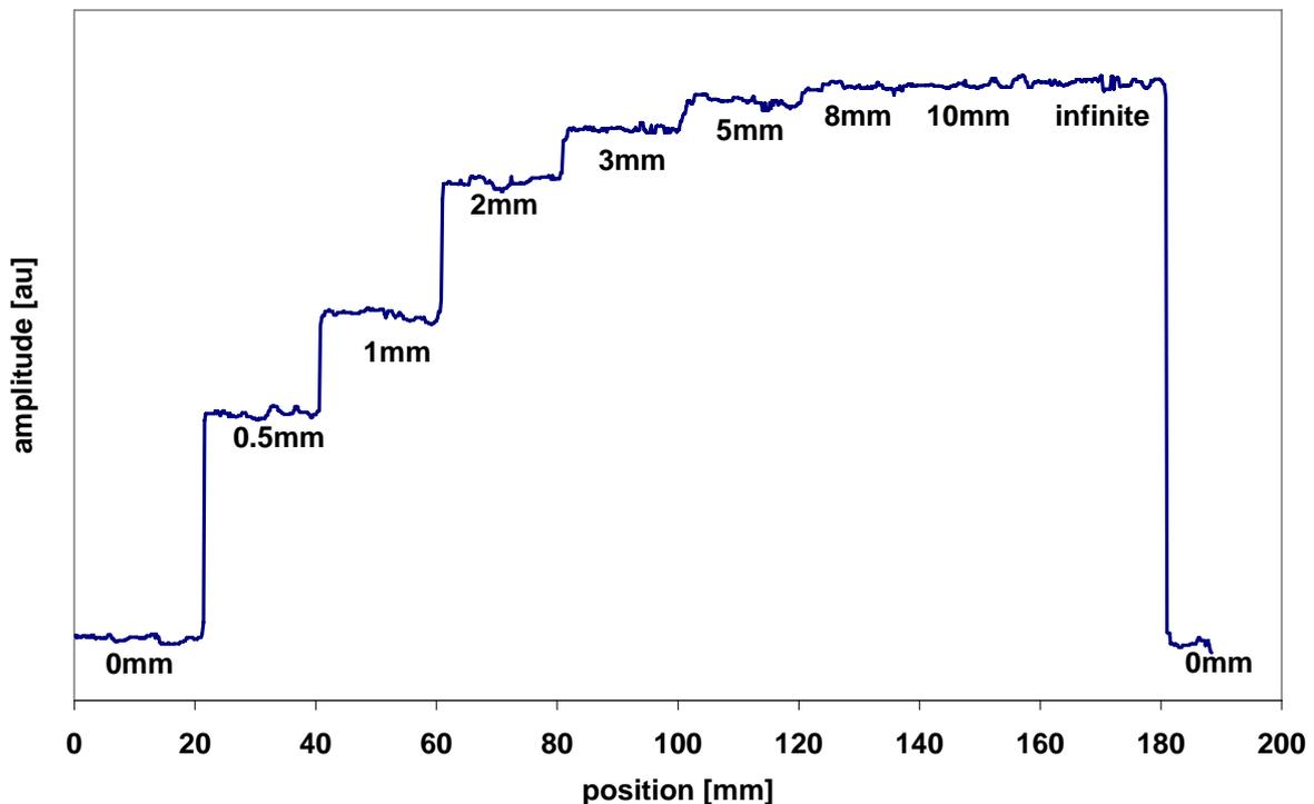
**Figure 7:** EC amplitude for different sensor lift-off
