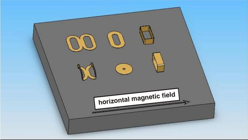
**Figure 4:** Investigated coil types: upper row, from left to right: butterfly coil, oval coil, rectangular coil (1); lower row: butterfly coil with angled return paths, spiral or pan-cake coil, rectangular coil (2)
