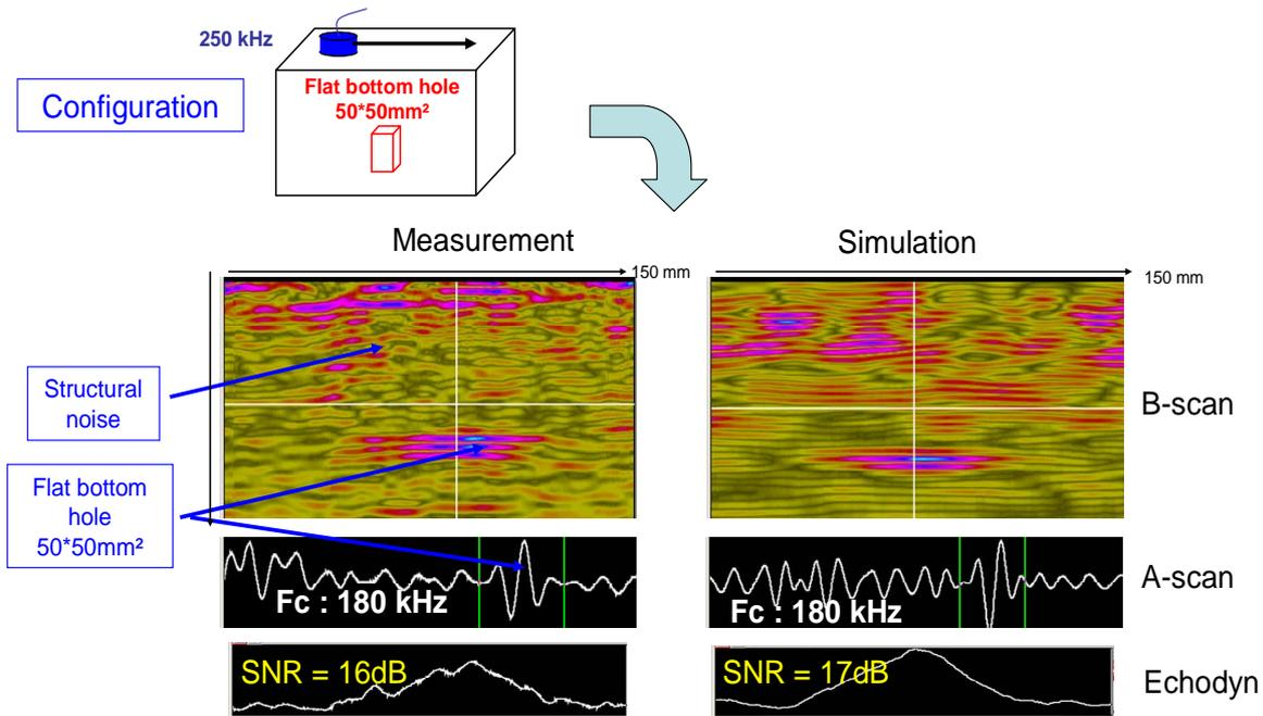
Fig. 4: Comparison of simulation to measurement for detection of a flat bottom hole by a mono element
