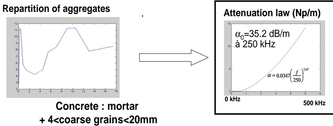
**Fig. 3:** Calculation of attenuation law from homogenization model
