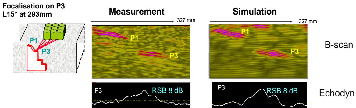
Fig. 5: Comparison of simulation to measurement for detection of a tilted defect by phased array
