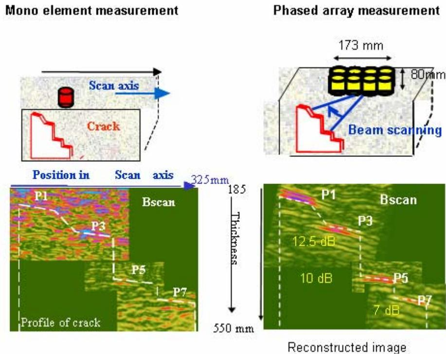
**Fig. 2:** Comparisons between mono-element measurement of the crack and the reconstructed Bscans images resulting from phased array measurements
