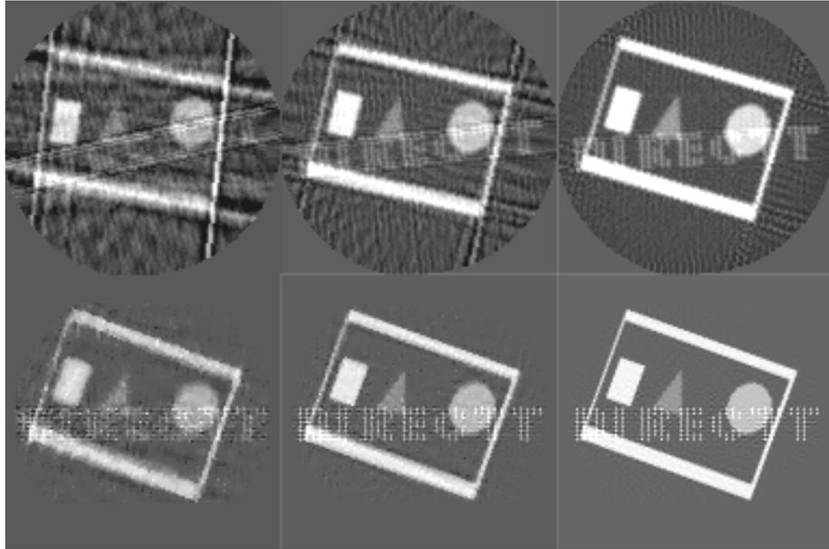
Fig. 6. Reconstruction results of both conventional (top) and DIRECTT (bottom) by reduced number of projections; the rotation intervals are constant over 180 degree, e.g. 15 projections of 12° separation, 30 x 6° and 60 x 3° (left to right).
