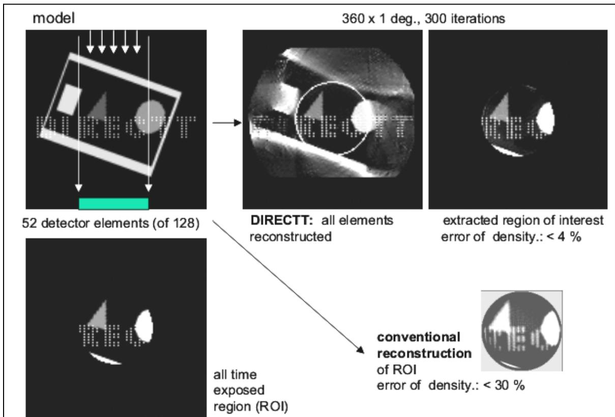
Fig. 8. Reconstruction from projections of a partial exposure (region of interest, ROI); model (left), ROI reconstructed by DIRECTT (top middle and right) and conventional (bottom, middle). Generally noise has no direct influence on the spatial resolution as the reconstruction procedure averages the sinogram data directly over the projection angles, not over the projection coordinate. Sharp contrasts are retained, although density noise occurs.
