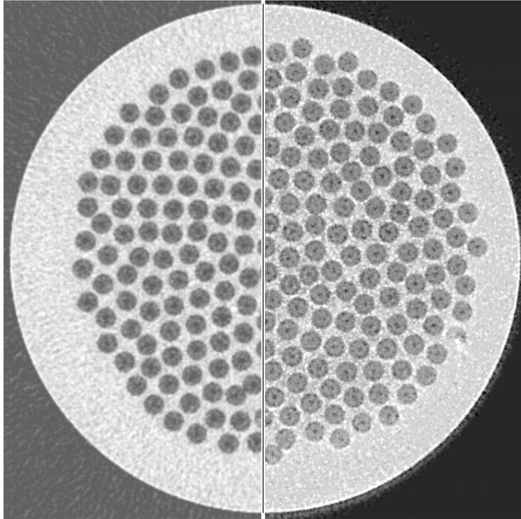
Fig. 10. Comparison of reconstructions from 39 keV parallel beam synchrotron radiation projections of 3.6 mm Ti/SiC MMC cylinder; left: conventional Fourier filtered back projection; right: DIRECTT
