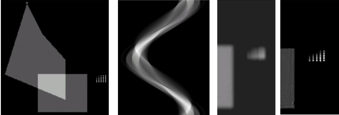
Fig. 9. Sub-pixel size resolution; model with 2x3 pixel grid, sinogram after 2 pixel binning, magnified section of Feldkamp reconstruction, DIRECTT reconstruction (from left to right)
