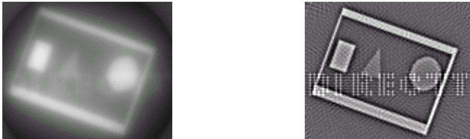
Fig. 5. DIRECTT reconstructions of box model after 1 iteration cycle; left : all weights; right all contrasts
