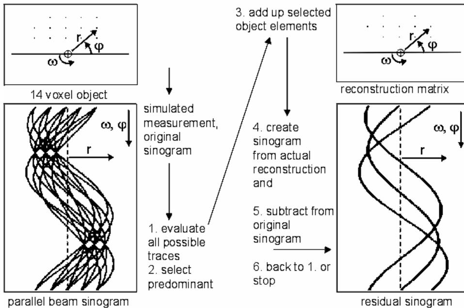
Fig. 1. Reconstruction principles of the iterative procedure
