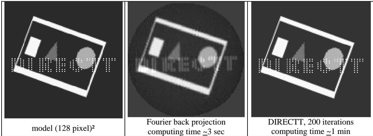
Fig.2. “box” phantom, Fourier filtered back projection and DIRECTT reconstruction.
