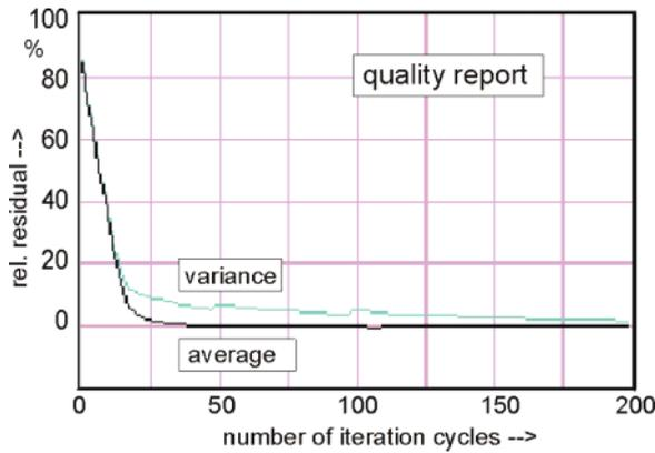
Fig. 4. Report on the reconstruction quality (of example in Fig. 3): average and variance of the residual sinograms over the number of iteration cycles.
