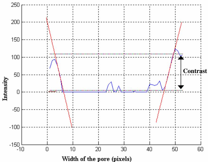
Figure 2: Intensity histogram of a pore of 70 $\mu$ m where the contrast is shown.
