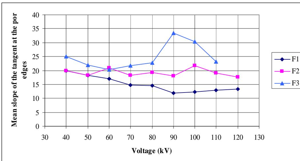
Figure 8: Influence of the acquisition parameters on the focus for a pore of 70 μm.
