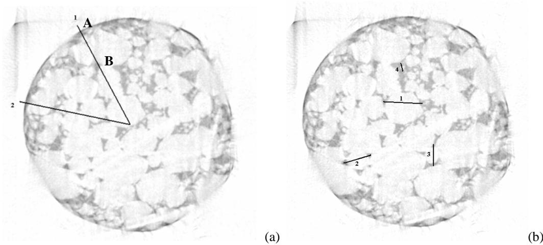
Figure 5: (a) The beam hardening effect is checked on path 1 and path 2, (b) the contrast and the focus are determined at pores 1 to 4, ranging from large to small pore size.
