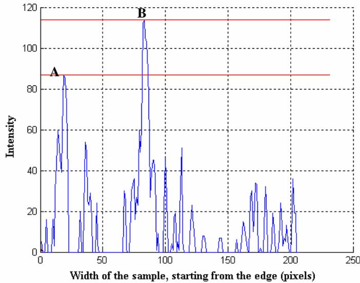
Figure 1: Profile of the material, generated at 110 kV and with a combination of an aluminium filter of 1 mm and a copper filter of 1 mm put right behind the source. Peak A represents the material at location A in figure 3a, peak B the material at location B.
