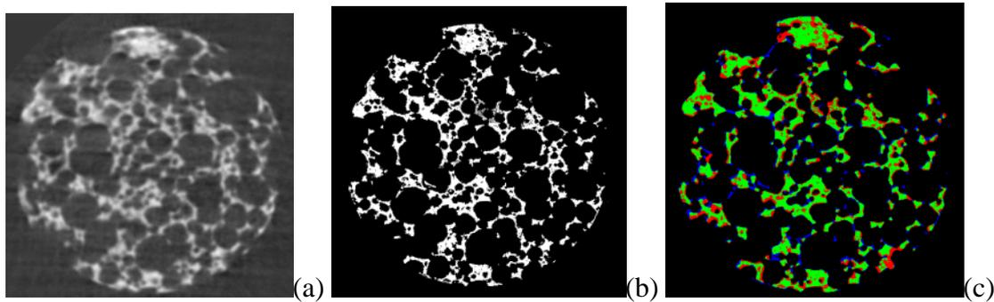
Figure 9: (a) Interpolated micro-CT image, (b) registered optical image and (c) overlap image of the sliced part Ti-A of a Ti sample.
