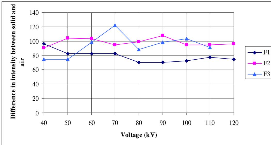
Figure 7: Influence of the acquisition parameters on the contrast for a pore of 70 μm
