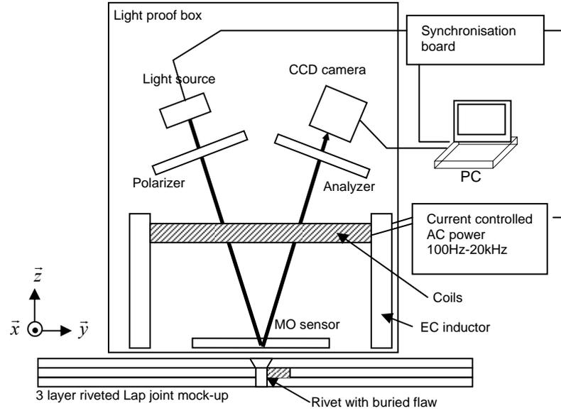
Figure 1. Schematic presentation of the eddy current imager
