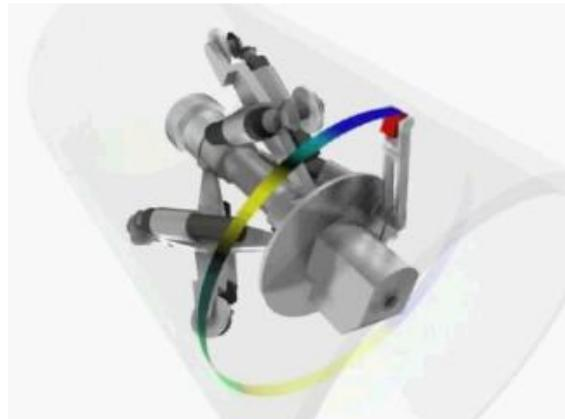
Fig. 7: Principle of crawler probe guiding system
