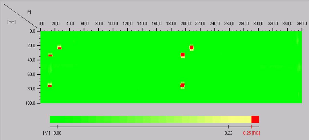
**Fig. 4:** Exemplary C-scan of the calibration body
