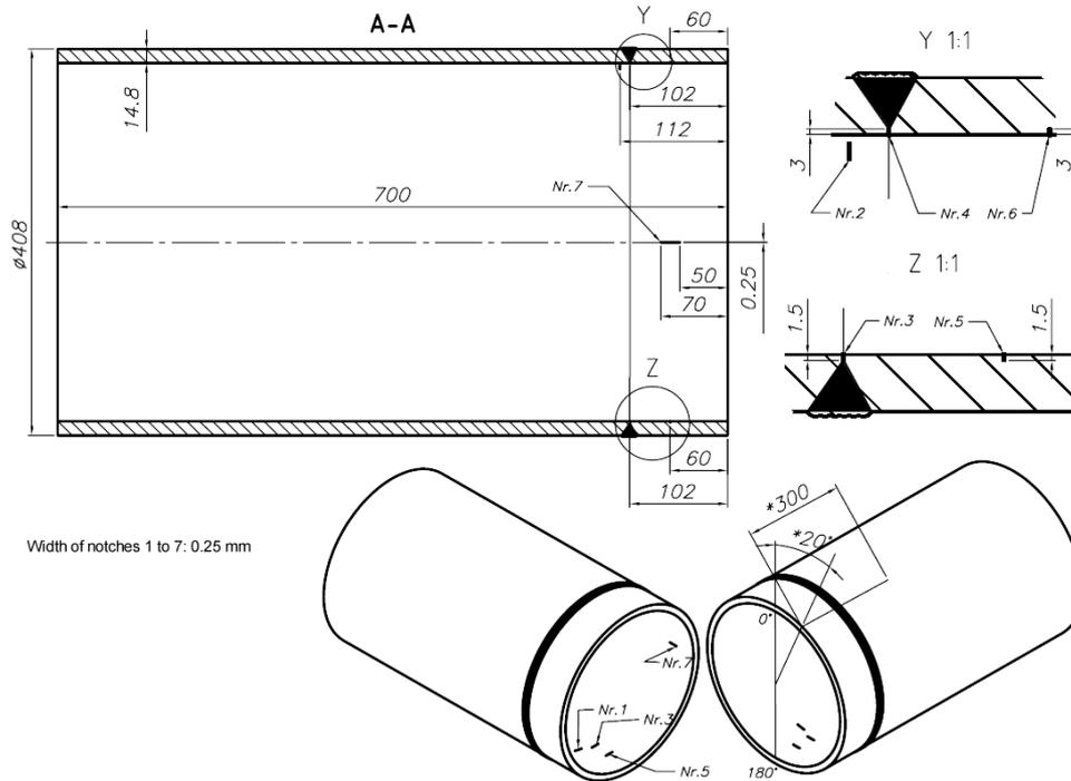
**Fig. 3:** Austenitic calibration body featuring a circumferential weld seam and seven calibration notches
