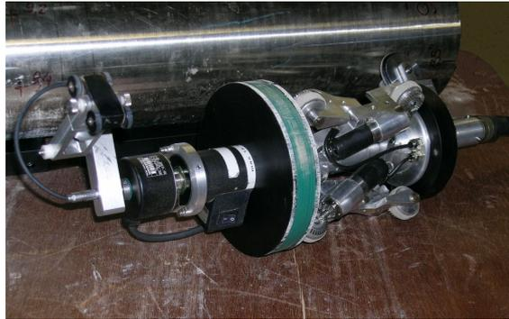
Fig. 6: Crawler with eddy current probes
