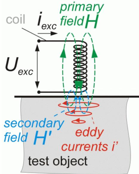
Fig. 1: Eddy current inspection system
