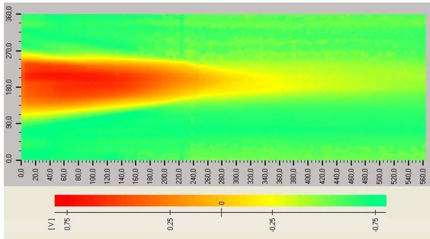
**Fig. 8:** C-scan of a pipe-inspection regarding wall-thickness reductions
