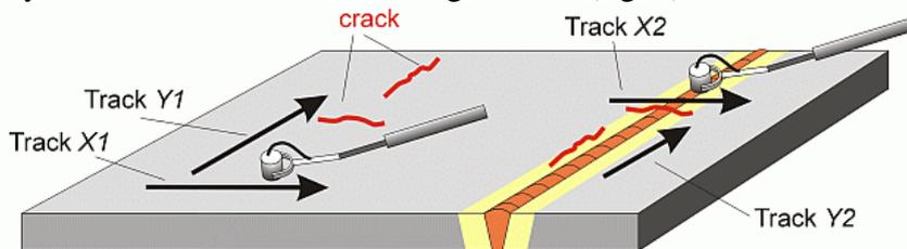
Fig. 2: Two-dimensional scanning of test object (left standard sheet, right welded sheets)
