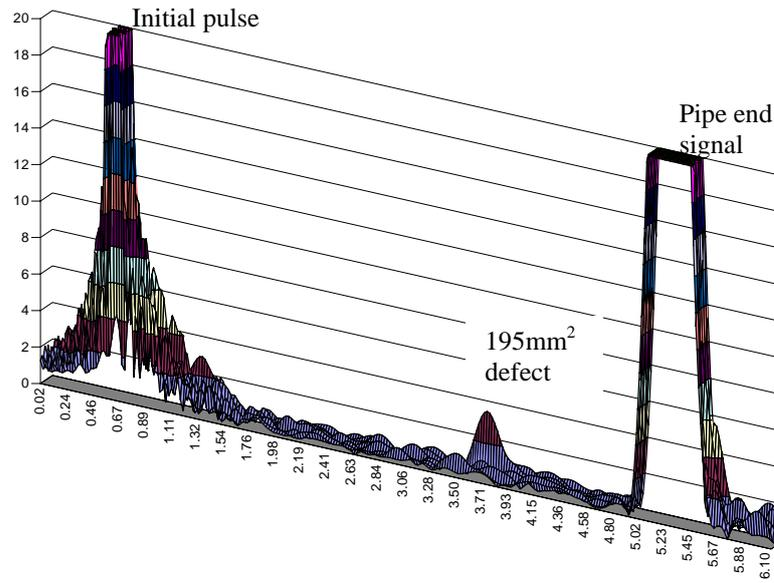
Fig. 4. Response from a 195mm<sup>2</sup> defect in a 10" (273mm) diameter pipe after focusing
