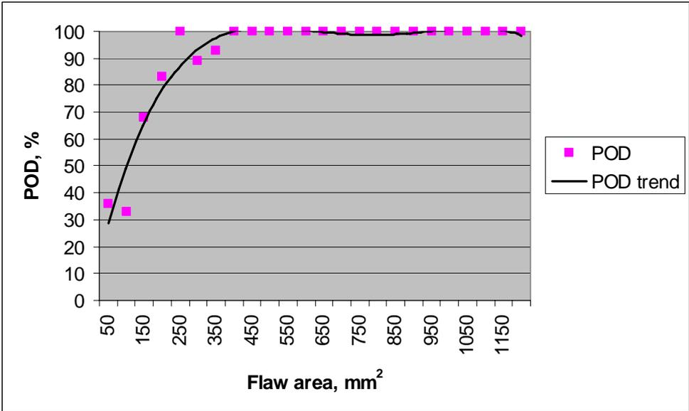
Fig. 1. Experimental probability of detection (PoD) for guided wave tests
