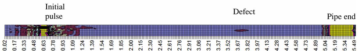
Fig.3. C-scan plot of 195mm<sup>2</sup> defect at the 12 o’clock position in a 10” pipe
