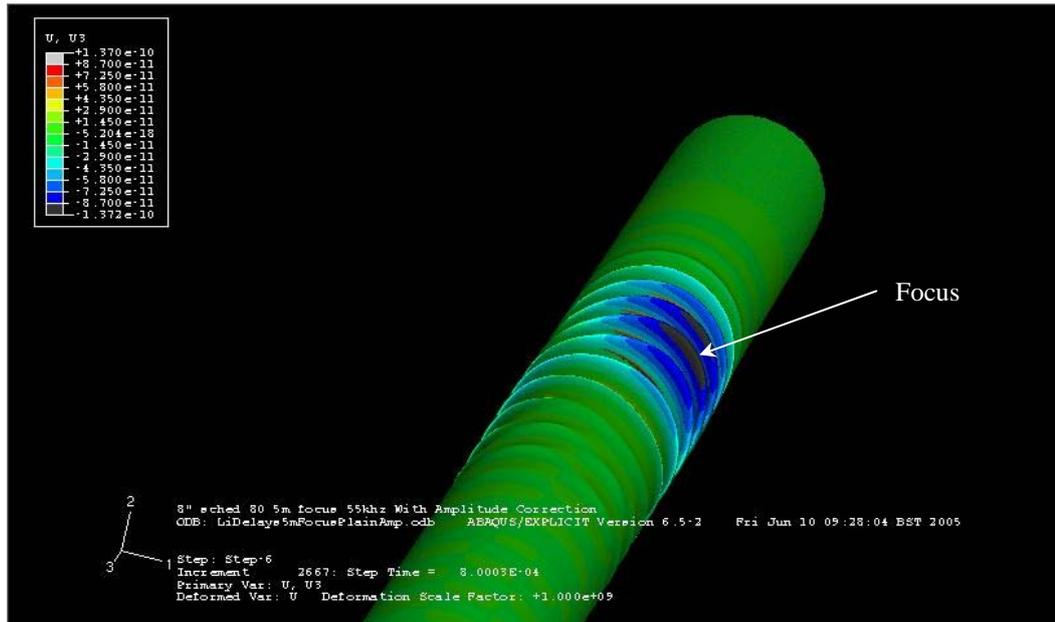
Fig. 2 Finite element model of the focus (at 45°) of ultrasonic guided waves in an 8” pipe
