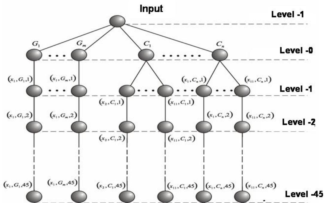
Fig. 3. Diagnostic tree for residual life evaluation.
