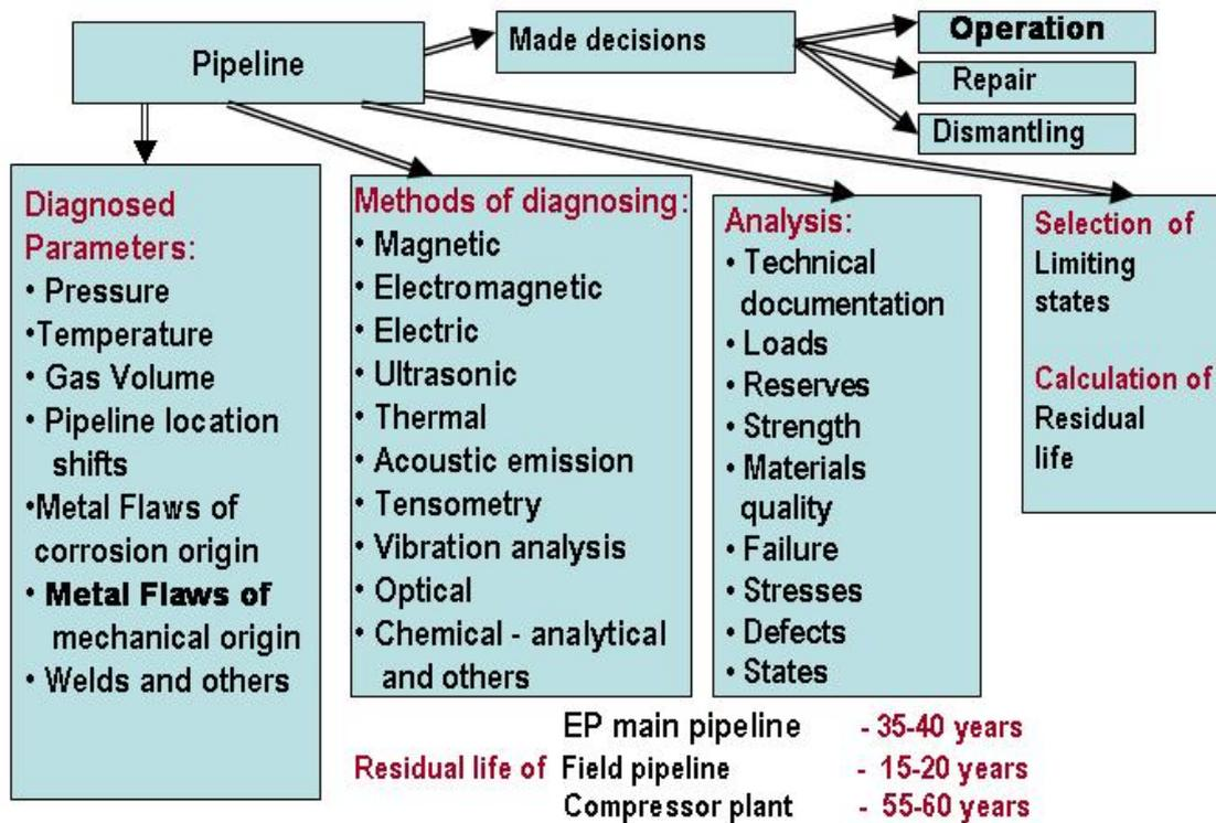
Fig. 5. Scheme of pipeline residual life evaluation.
