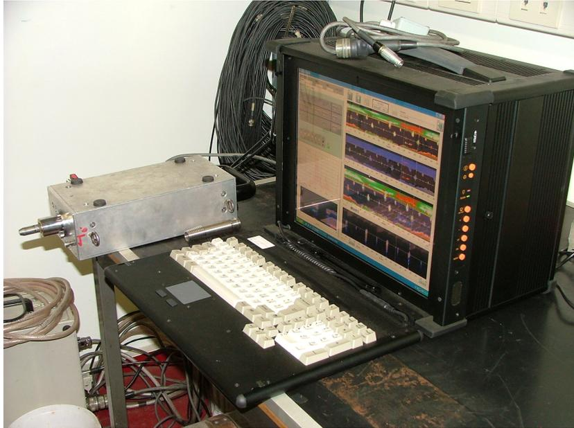
Fig. 5: Hiscan system with bore probe
