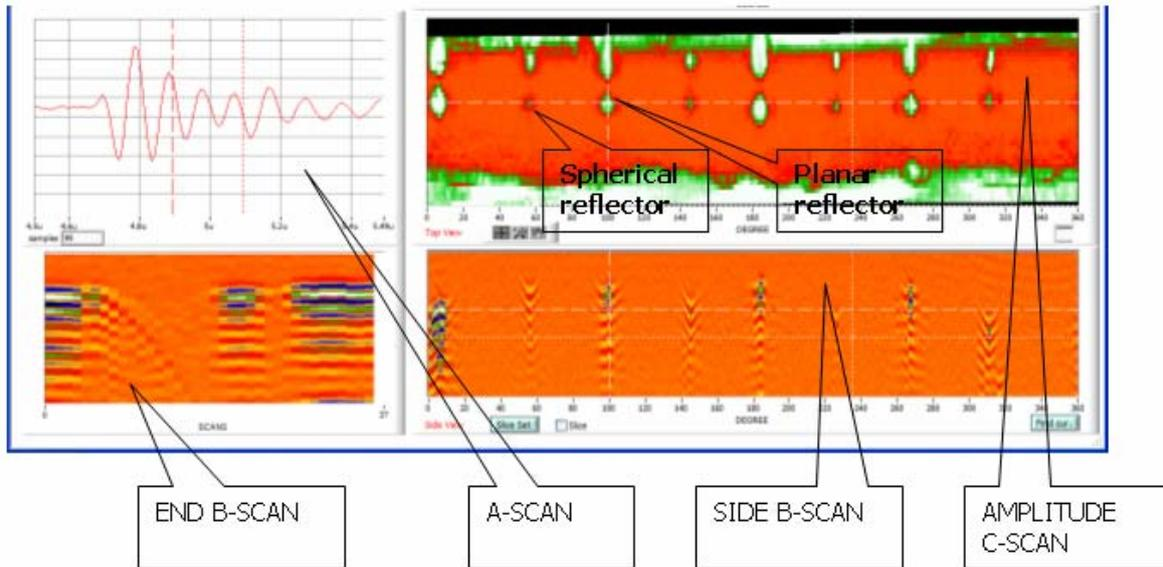
Fig. 7: Typical geometrical reconstruction
