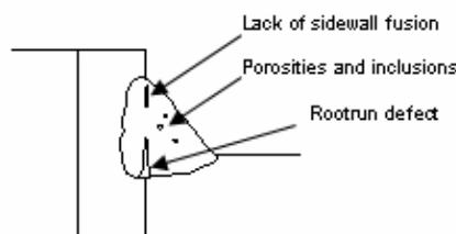
Fig. 3 Typical defects
