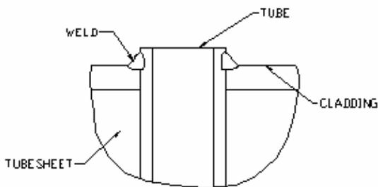
Fig. 1 Tube to tubesheet weld scheme
