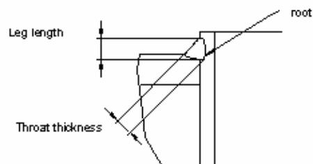
Fig. 2 Geometrical weld features
