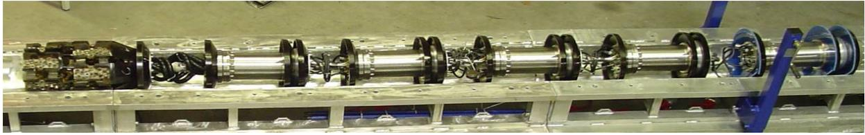
Figure 2 – 10-inch Crack Detection Tool
